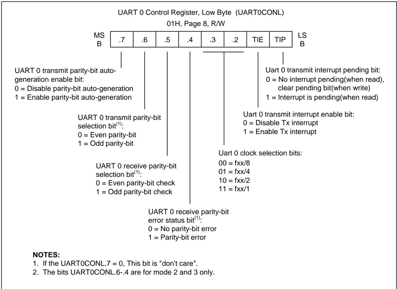
**Figure 19-2 UART 0 Low Byte Control Register (UART0CONL)**
