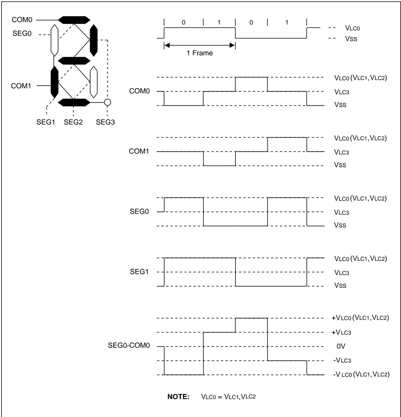
Figure 15-11 LCD Signal Waveforms (1/2 Duty, 1/2 Bias)
