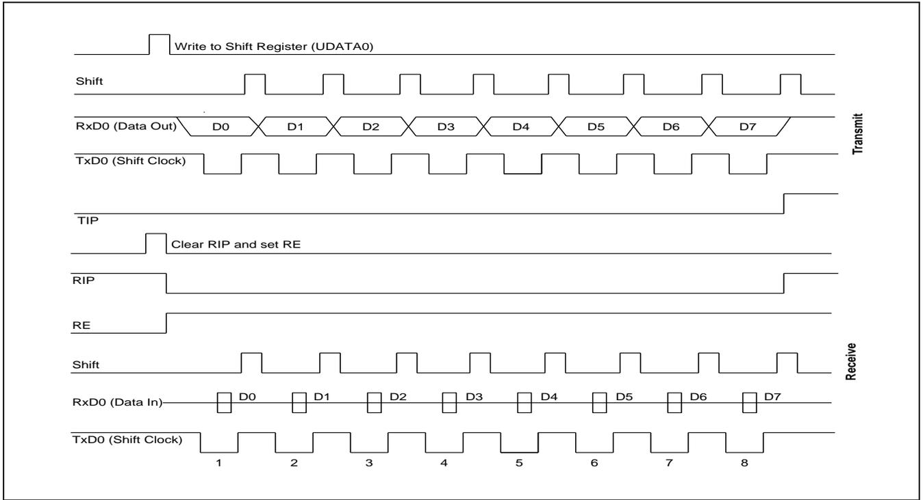
Figure 19-6 Timing Diagram for Serial Port Mode 0 Operation
