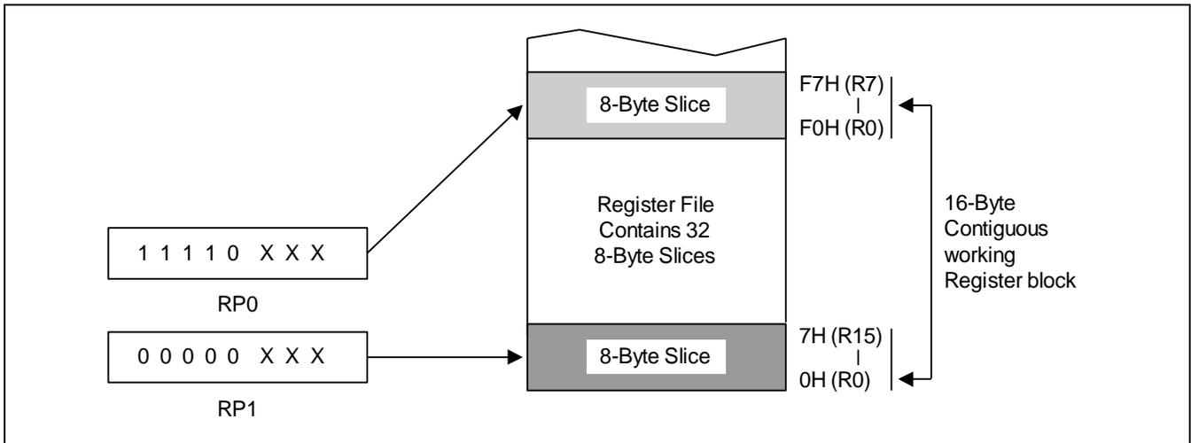
Figure 2-8 Non-Contiguous 16 Byte Working Register Block
