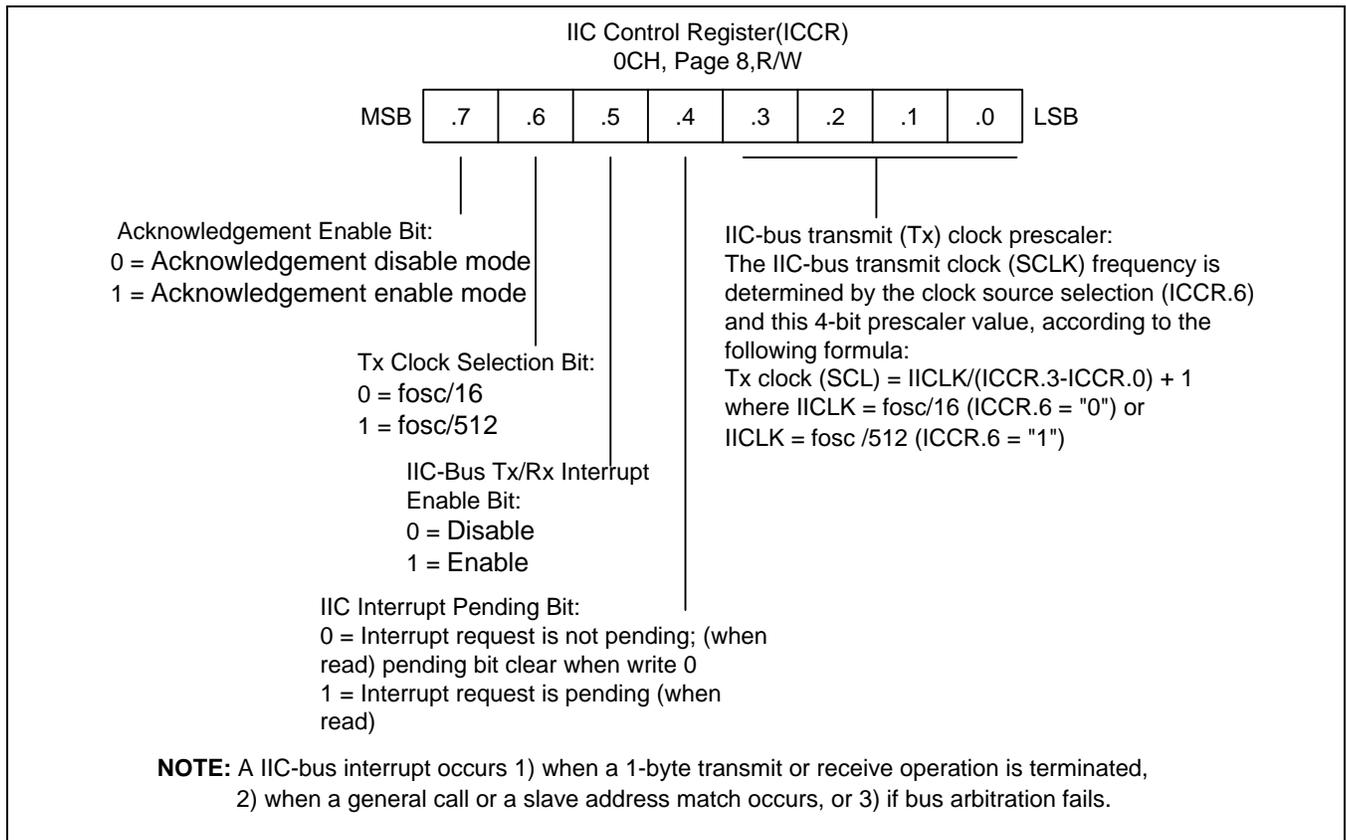
**Figure 18-1 Multi-Master I2C Bus Control Register (ICCR)**
