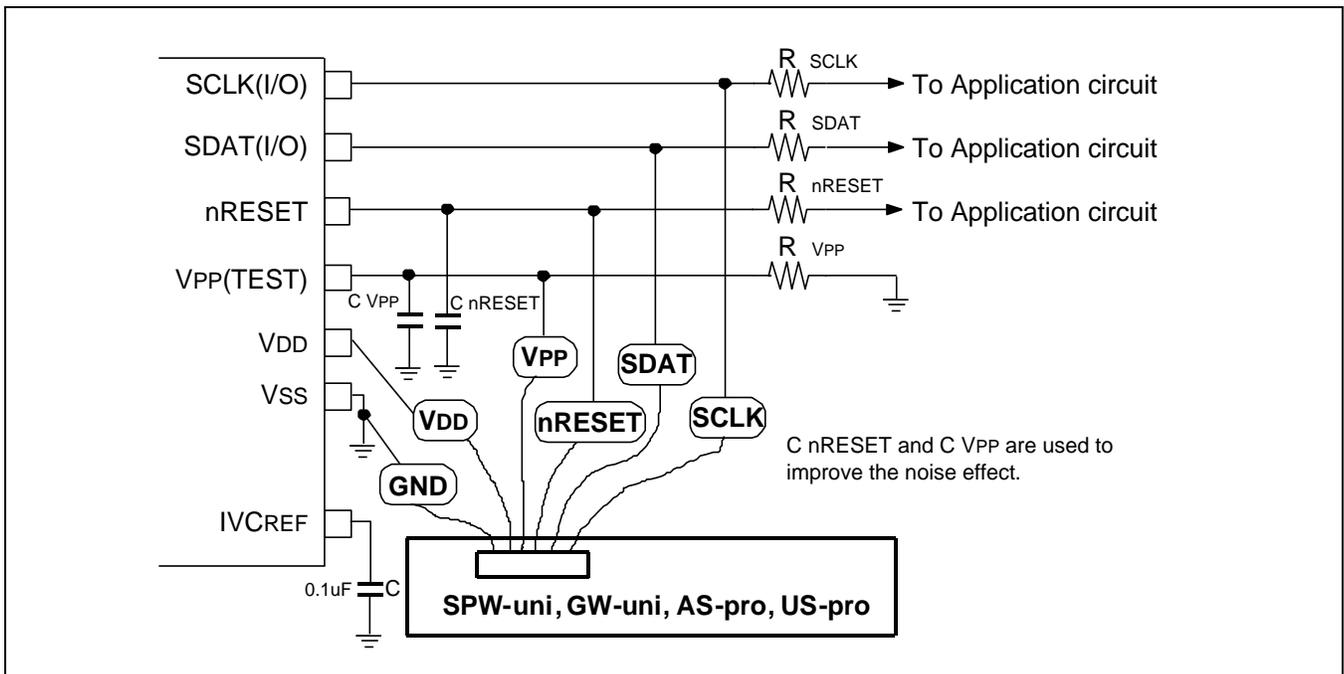
**Figure 25-3 PCB Design Guide for on Board Programming**
