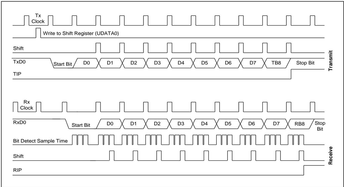
**Figure 19-9 Timing Diagram for Serial Port Mode 3 Operation**
