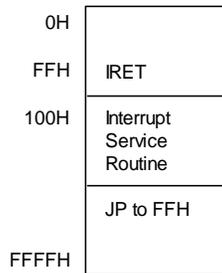
**NOTE:** In this fast interrupt example in the figure above, if the last instruction is not a jump to IRET, you must pay attention to the order of the last two instructions. The IRET cannot be immediately preceded by a clearing of the interrupt status (as with a reset of the IPR register).
