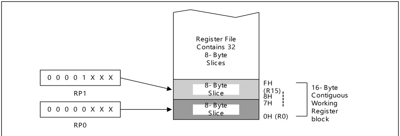
**Figure 2-7 Contiguous 16 Byte Working Register Block**
