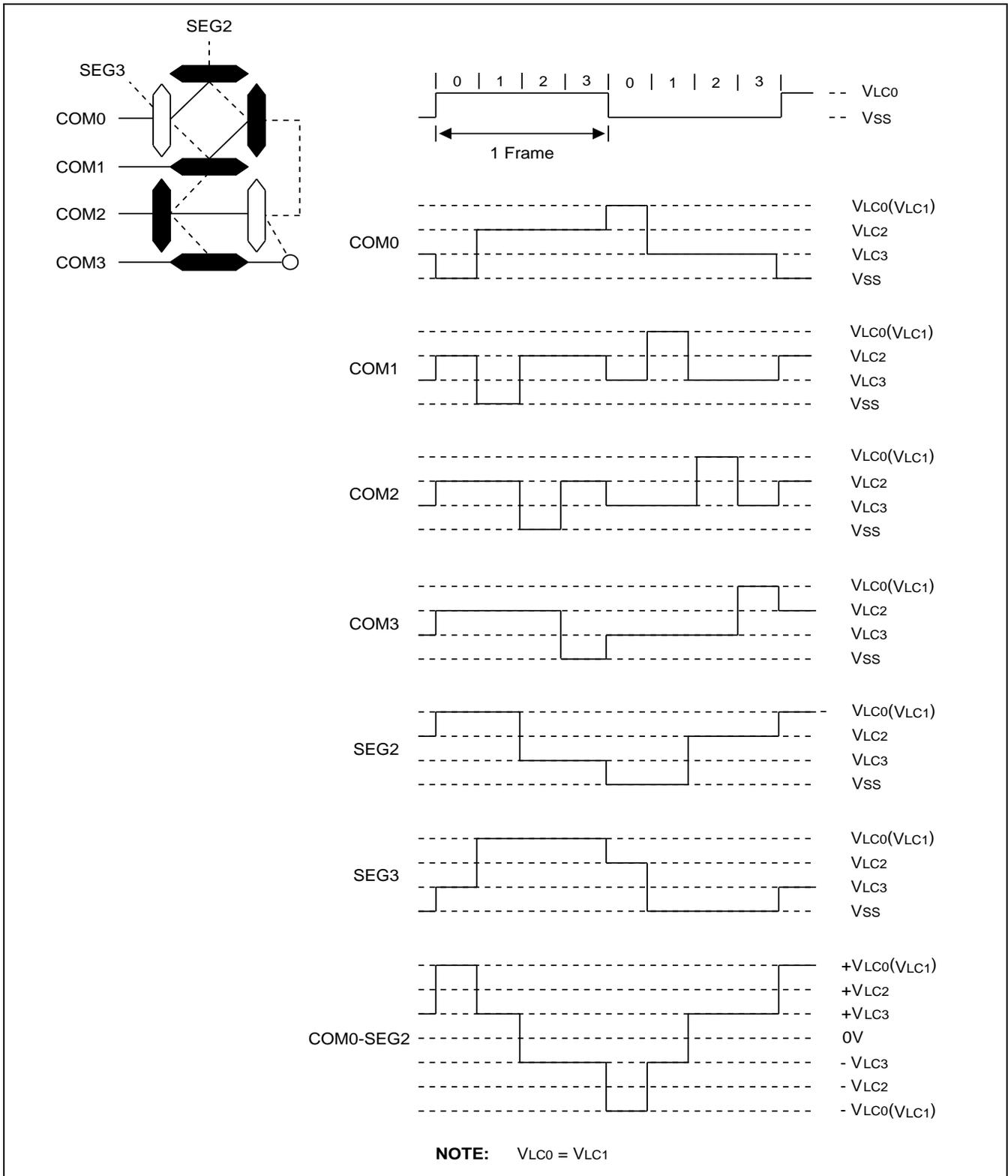
**Figure 15-13 LCD Signal Waveforms (1/4 Duty, 1/3 Bias)**
