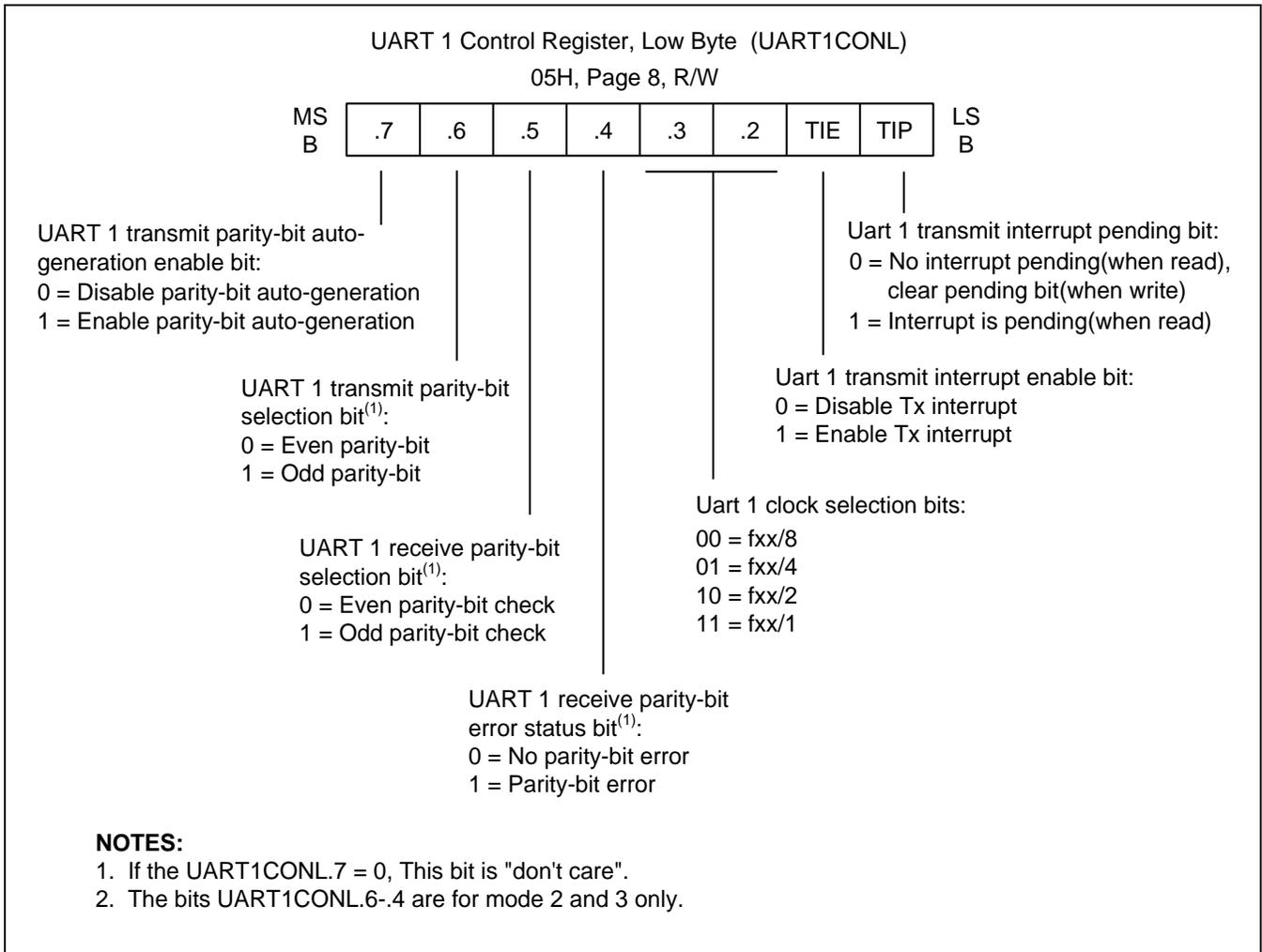
**Figure 20-2 UART 1 Low Byte Control Register (UART1CONL)**
