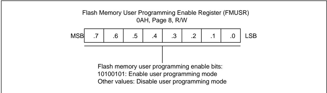
**Figure 21-2 Flash Memory User Programming Enable Register (FMUSR)**
