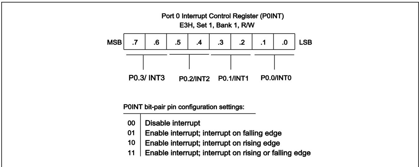
Figure 9-3 Port 0 Interrupt Control Register (POINT)
