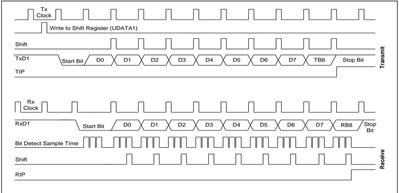
Figure 20-8 Timing Diagram for Serial Port Mode 2 Operation
