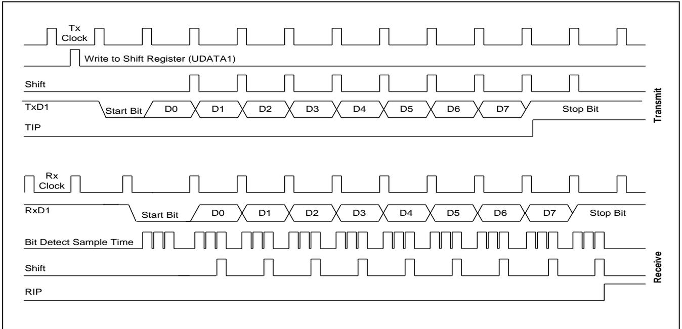
**Figure 20-7 Timing Diagram for Serial Port Mode 1 Operation**
