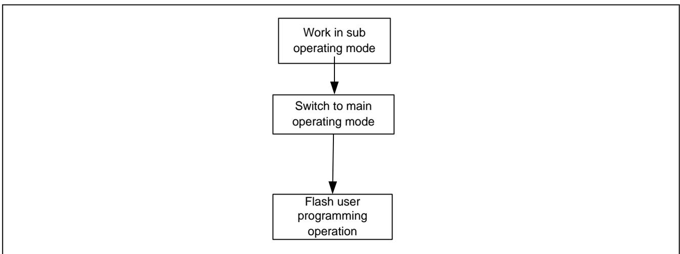
**Figure 21-7 Flash Operation Sequence in Sub Operating Mode**
