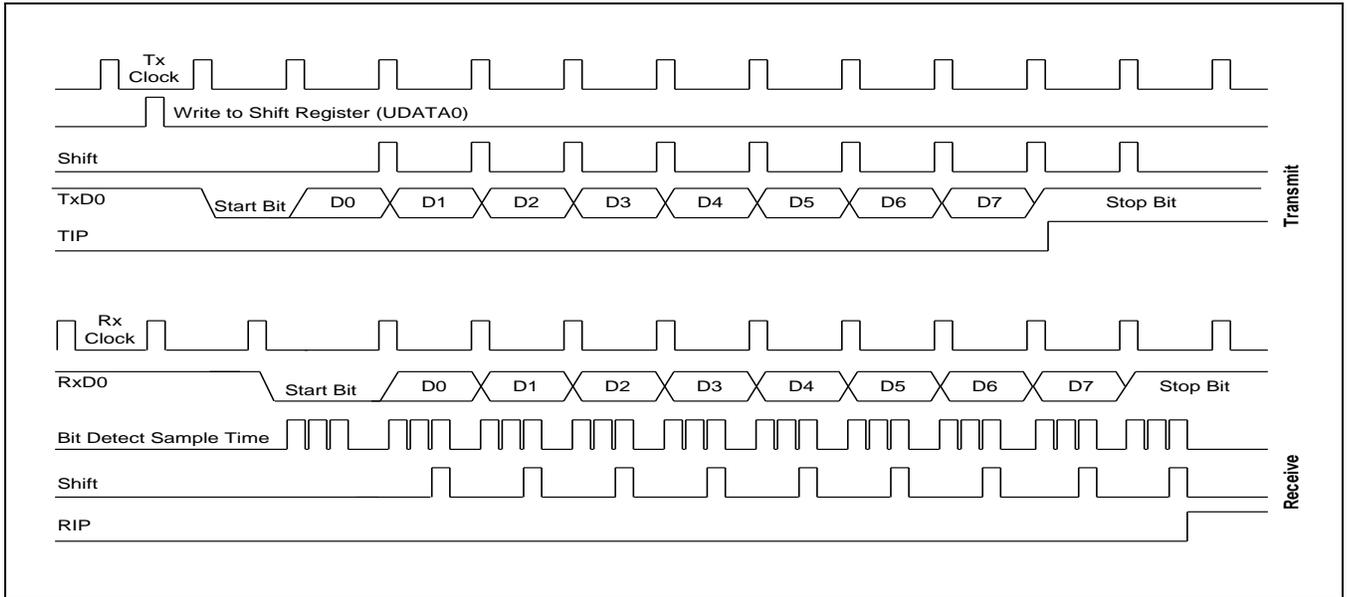
Figure 19-7 Timing Diagram for Serial Port Mode 1 Operation
