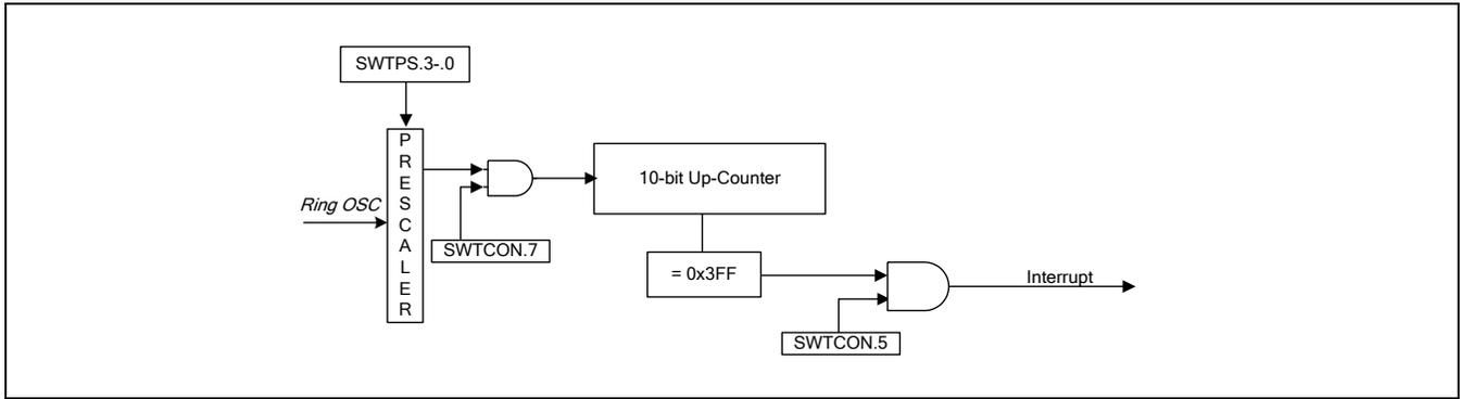
**Figure 12-2 Stop Wake-Up Timer Functional Block Diagram**
