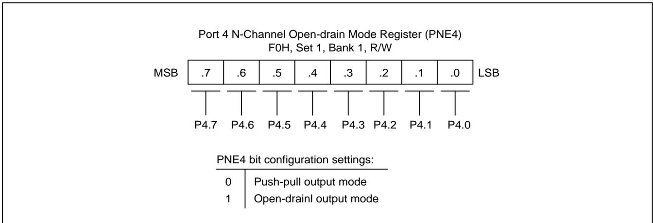
**Figure 9-17 Port 4 N-Channel Open-Drain Mode Register (PNE4)**
