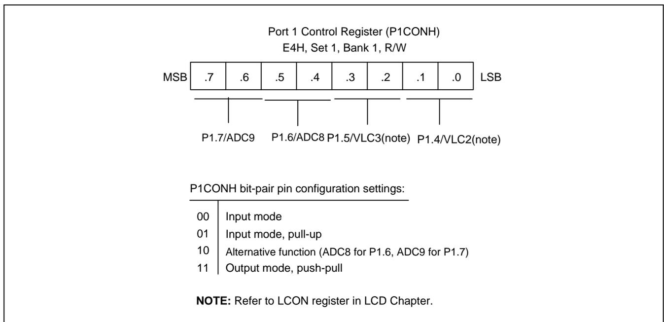
**Figure 9-4** Port 1 Control Register High Byte
