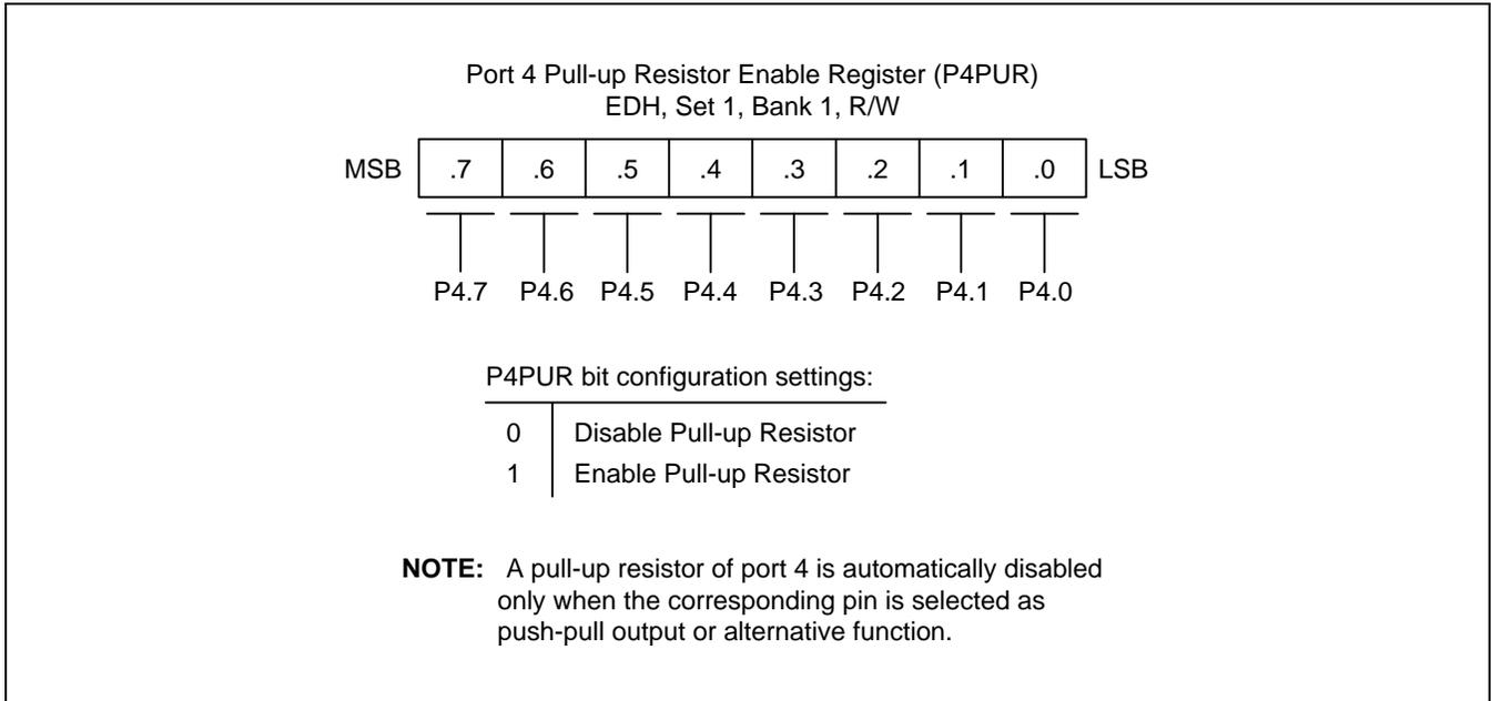
**Figure 9-16 Port 4 Pull-Up Resistor Enable Register (P4PUR)**
