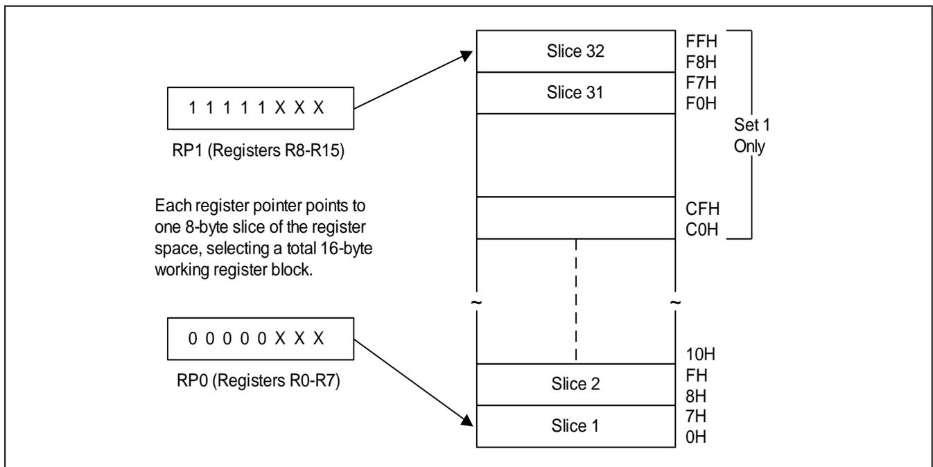
**Figure 2-6 8 Byte Working Register Areas (Slices)**
