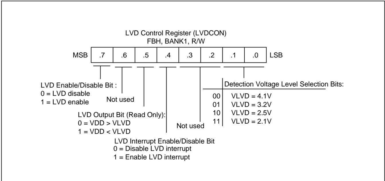
Figure 22-3 Flash Low Voltage Detect Control Register (LVDCON)
