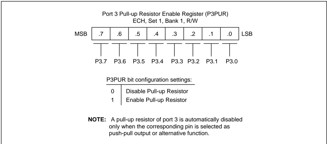
Figure 9-12 Port 3 Pull-Up Resistor Enable Register (P3PUR)
