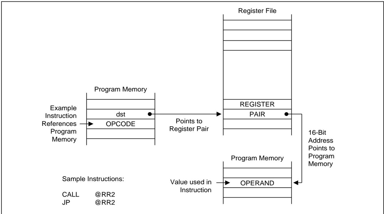
Figure 3-4 Indirect Register Addressing to Program Memory
