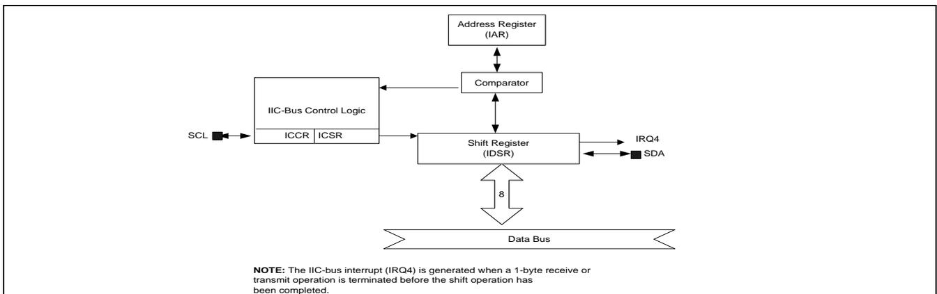
**Figure 18-4 Multi-Master I2C Bus Address Register (IAR)**
