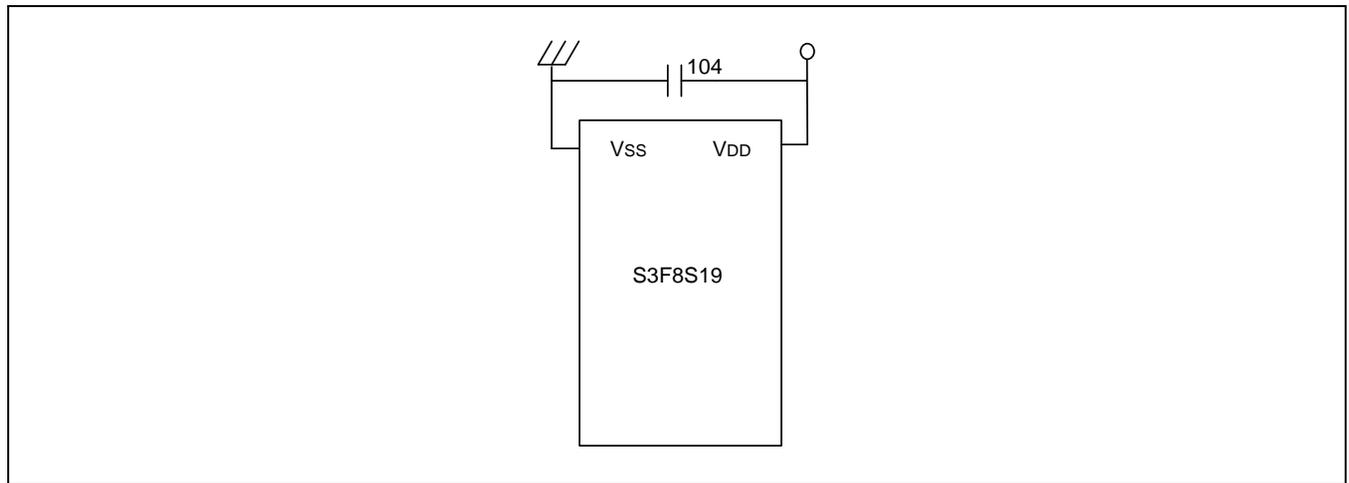
**Figure 23-6 The Circuit Diagram to Improve EFT Characteristics**
