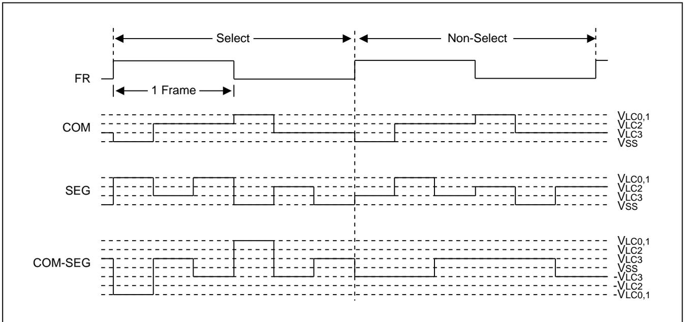
Figure 15-10 Select/No-Select Signal in 1/3 Duty, 1/3 Bias Display Mode
