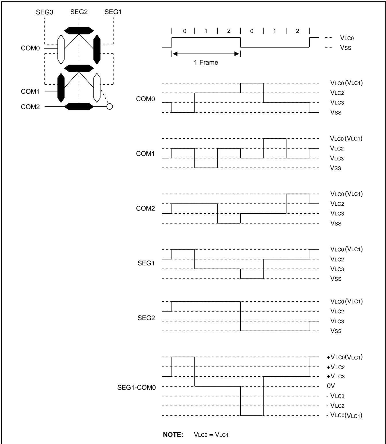
**Figure 15-12 LCD Signal Waveforms (1/3 Duty, 1/3 Bias)**
