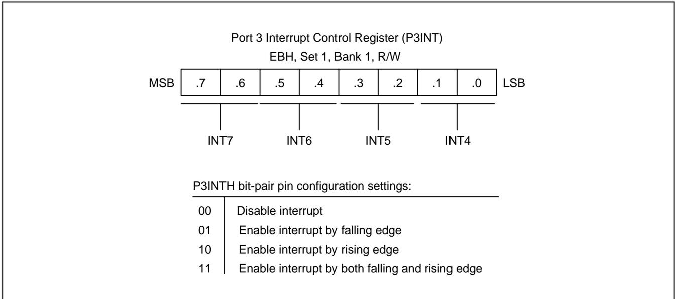
**Figure 9-10 Port 3 Interrupt Control Register (P3INT)**
