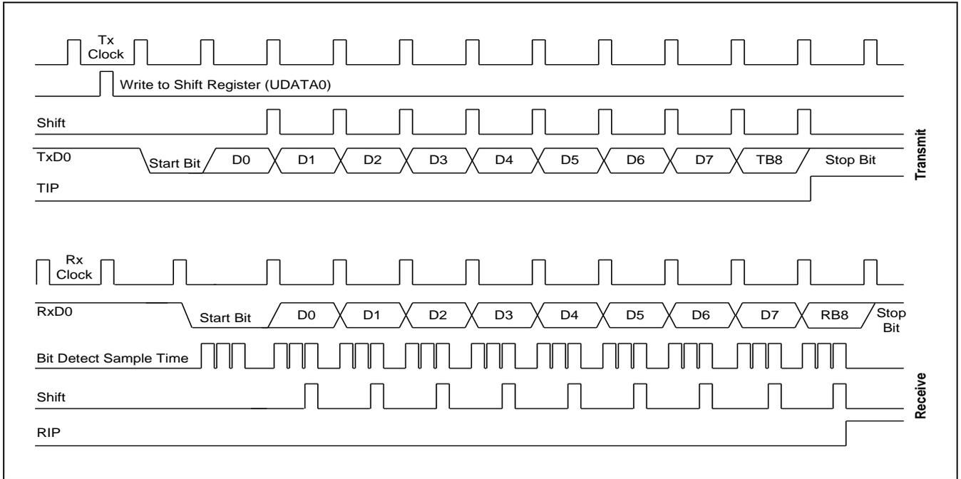
Figure 19-8 Timing Diagram for Serial Port Mode 2 Operation
