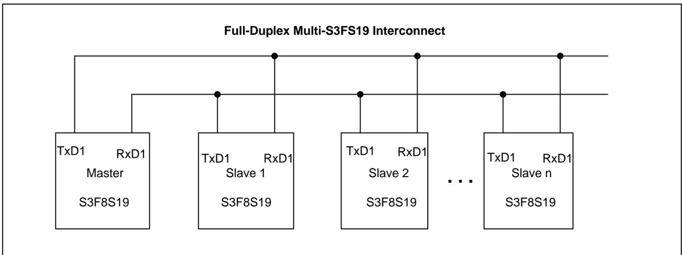
**Figure 20-10 Connection Example for Multiprocessor Serial Data Communications**
