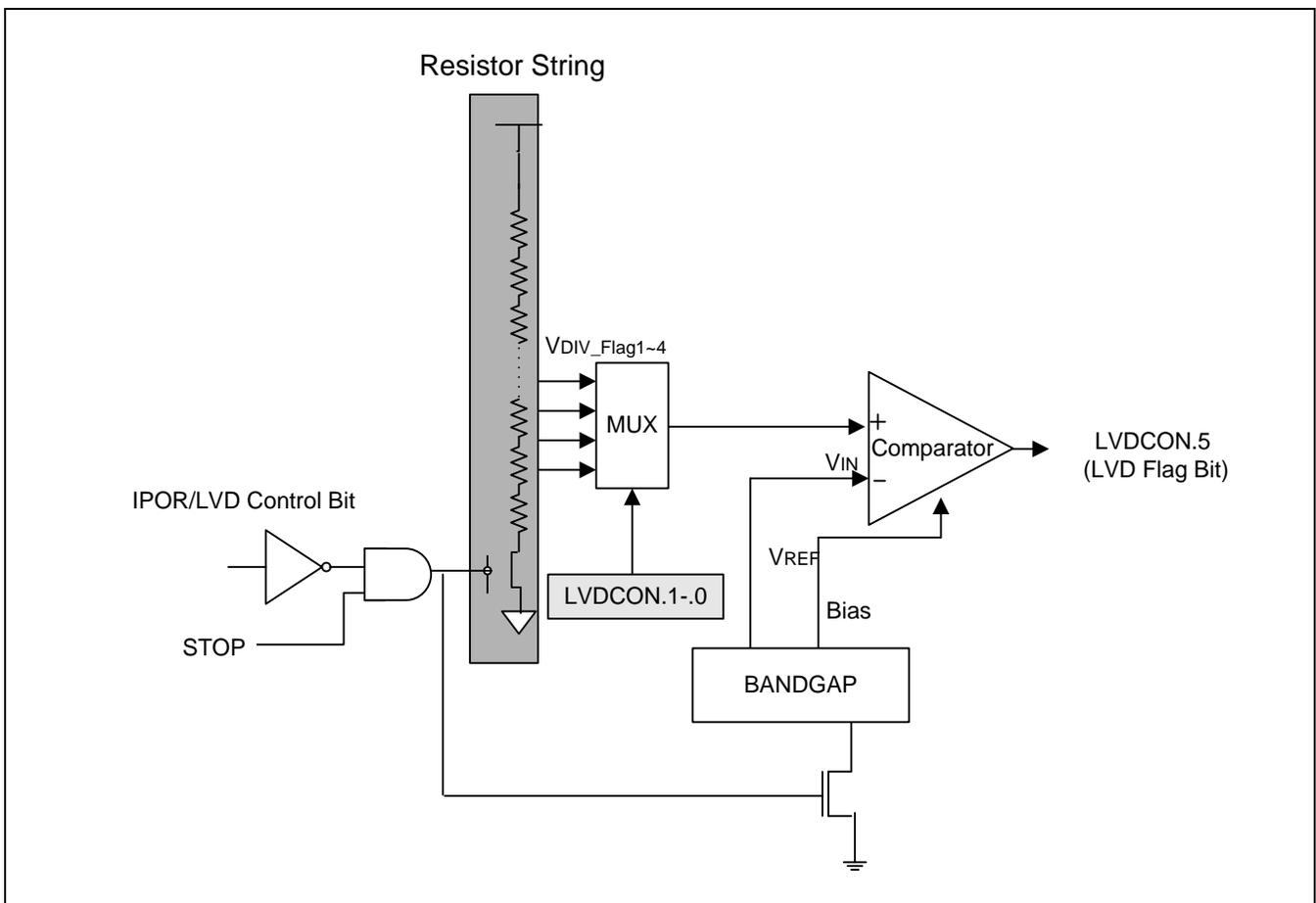
**Figure 22-2 Low Voltage Detect (LVD) Block Diagram**
