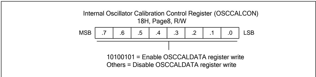
**Figure 7-5 Internal Oscillator Calibration Control Register (OSCCALCON)**
