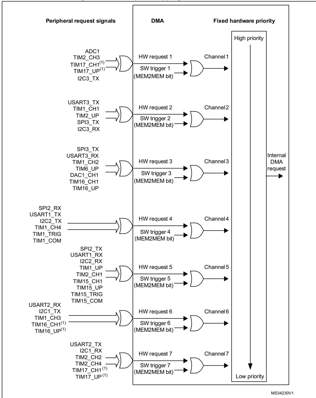
1. DMA request mapped on this DMA channel only if the corresponding remapping bit is set in *SYSCFG configuration register 1 (SYSCFG\_CFGR1)* and *SYSCFG register map*.
