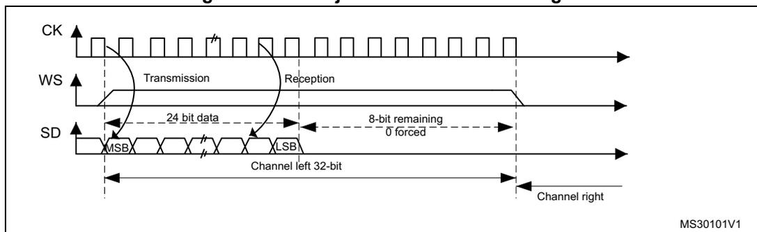
**Figure 367. MSB justified 16-bit extended to 32-bit packet frame**
