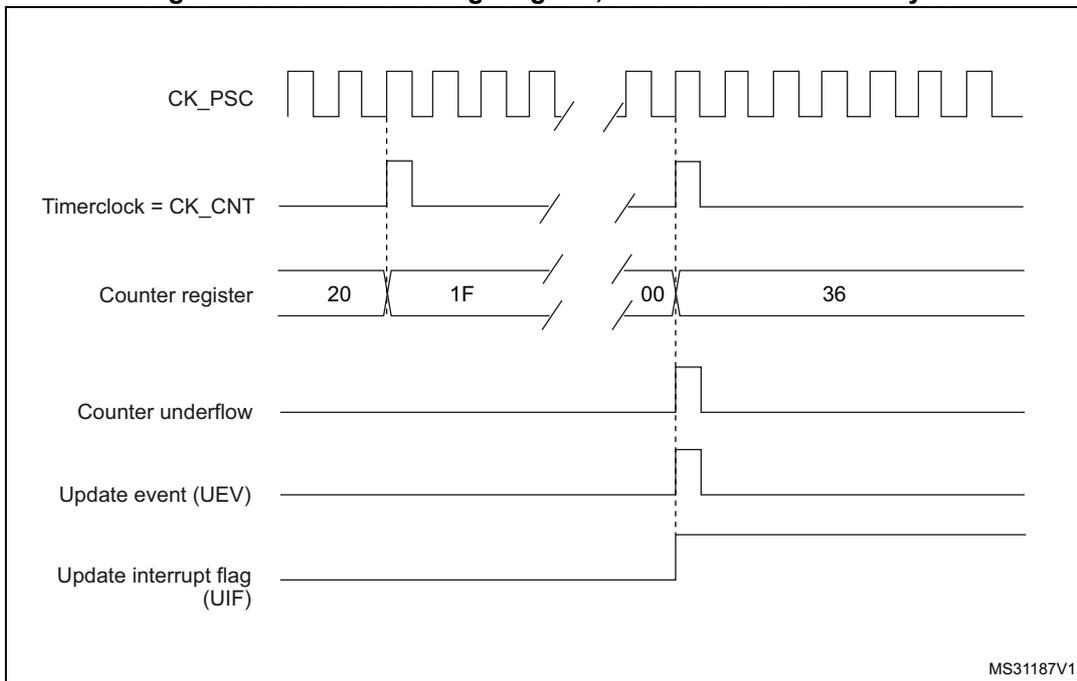
**Figure 145. Counter timing diagram, update event when repetition counter is not used**
