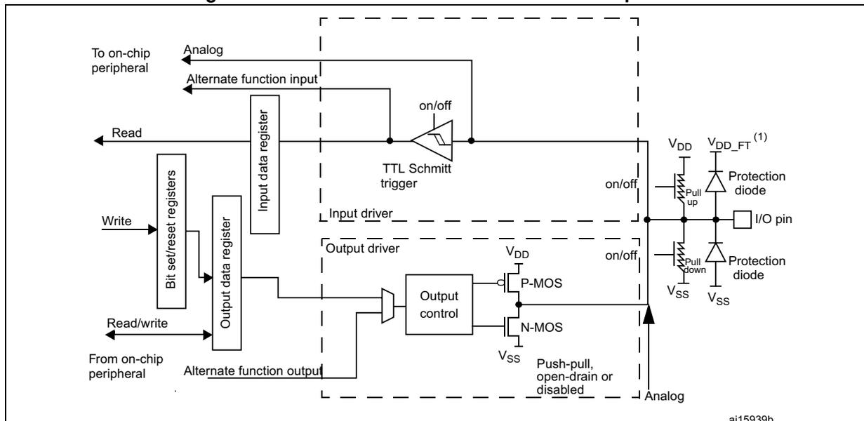
1.  $V_{DD\_FT}$  is a potential specific to 5-Volt tolerant I/Os and different from  $V_{DD}$ .
