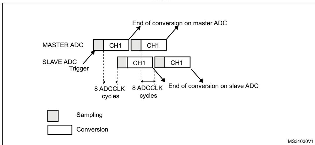
**Figure 99. Interleaved mode on 1 channel in single conversion mode: dual ADC mode**
