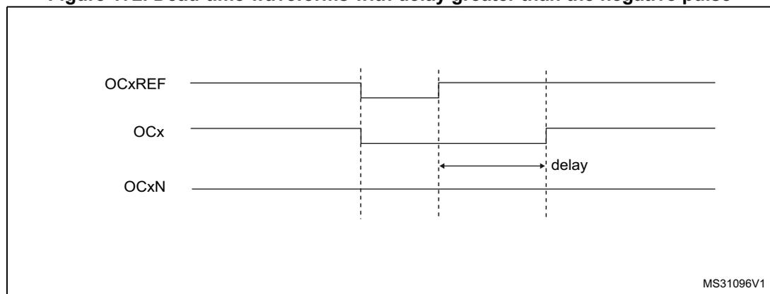
**Figure 173. Dead-time waveforms with delay greater than the positive pulse**
