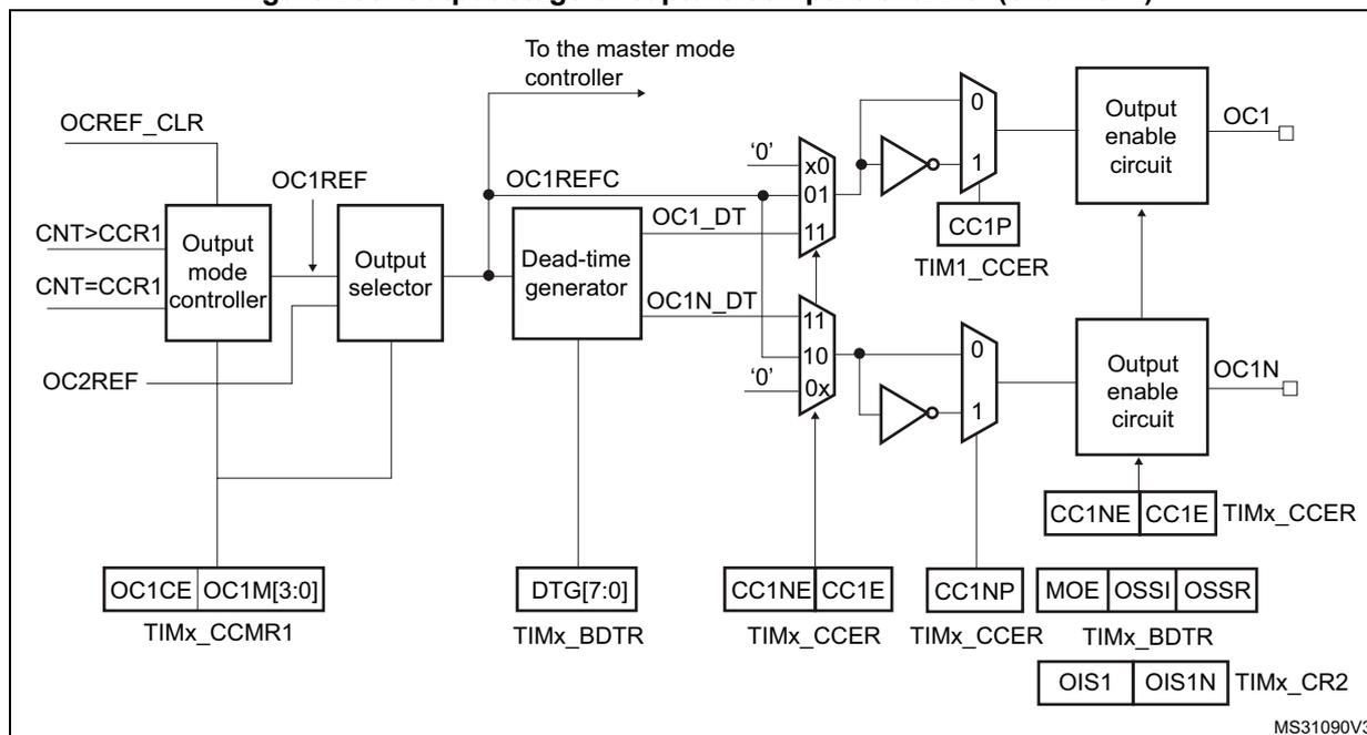
Figure 256. Output stage of capture/compare channel (channel 2 for TIM15)
