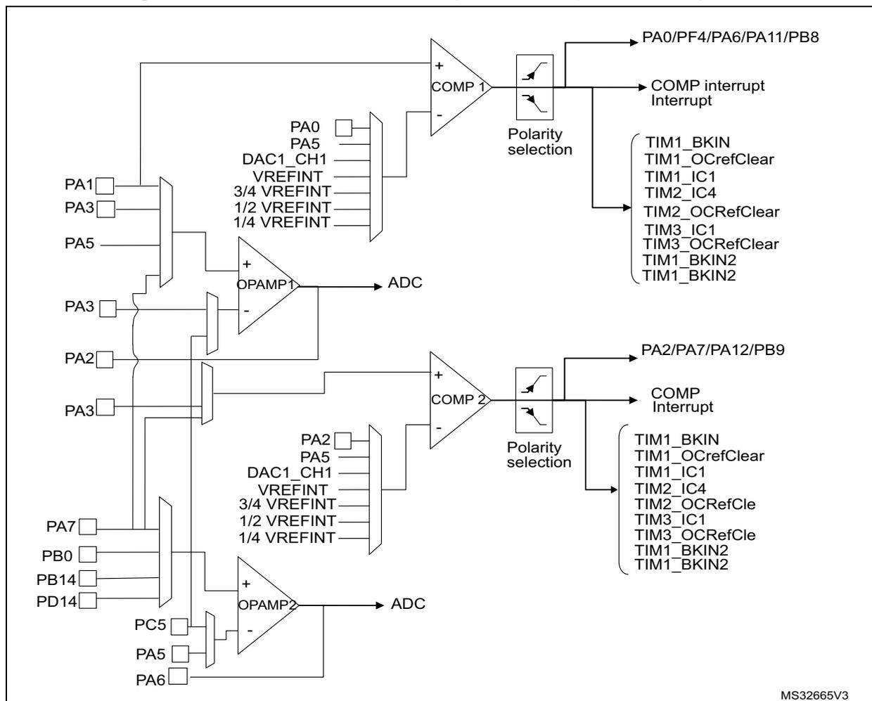
Figure 121. STM32F302x6/8 comparator and operational amplifier connections
