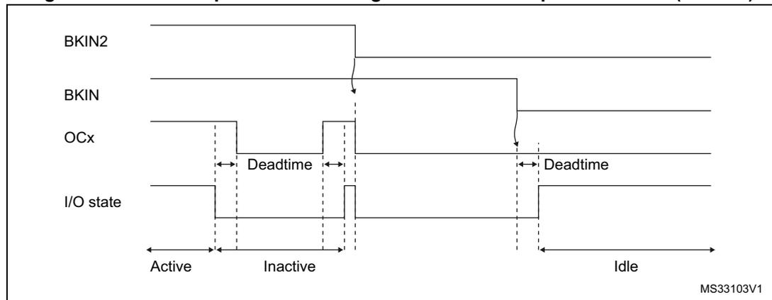
Figure 176. PWM output state following BKIN assertion (OSSI=0)
