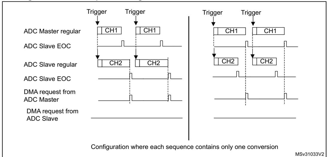
**Figure 107. DMA requests in interleaved mode when MDMA=0b10**
