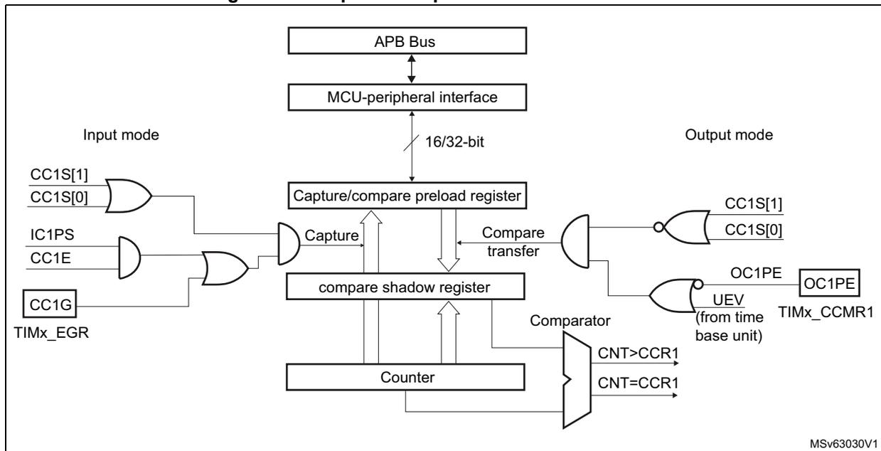
Figure 255. Output stage of capture/compare channel (channel 1)
