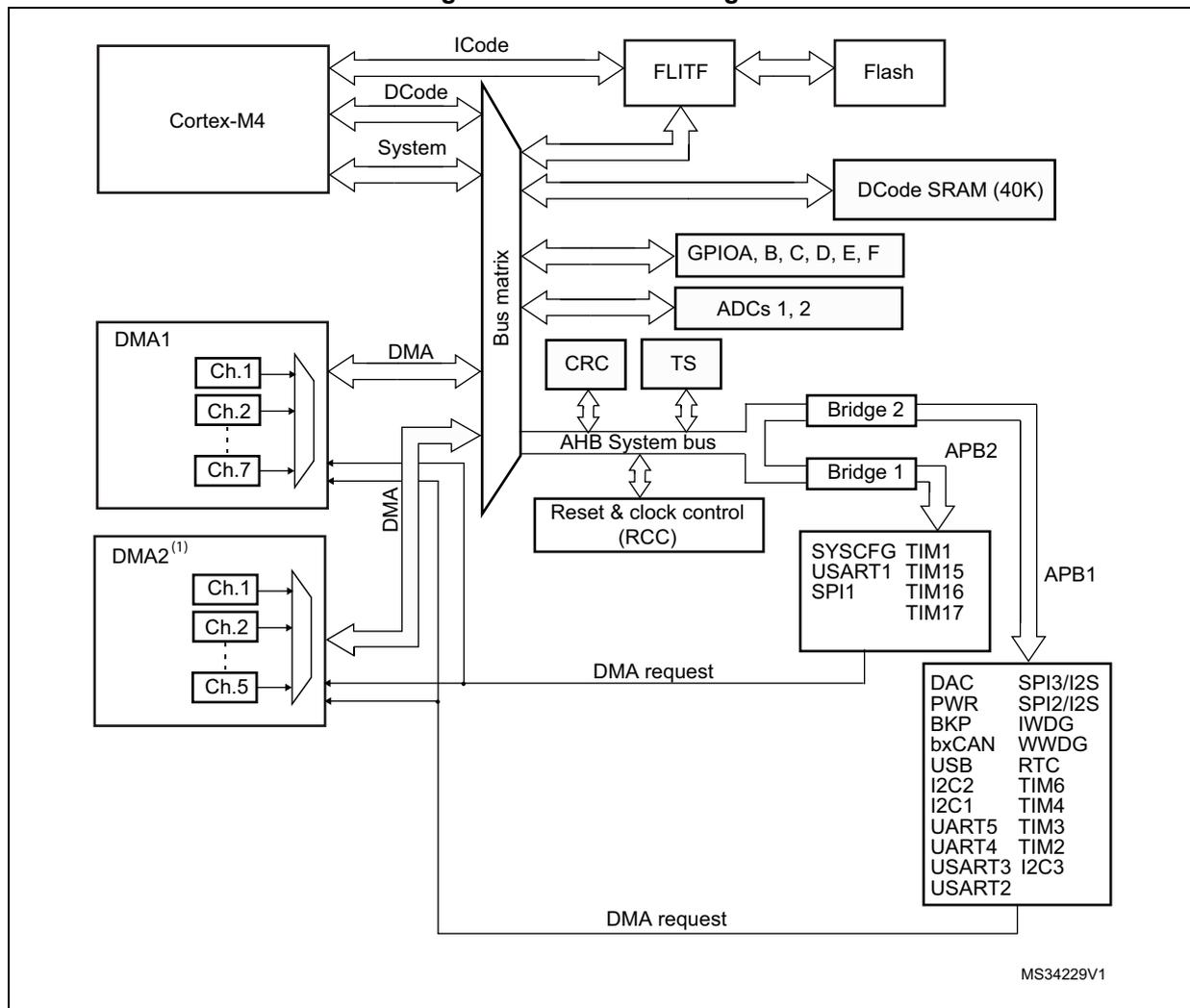
The DMA controller performs direct memory transfer by sharing the AHB system bus with other system masters. The bus matrix implements round-robin scheduling. DMA requests may stop the CPU access to the system bus for a number of bus cycles, when CPU and DMA target the same destination (memory or peripheral).
