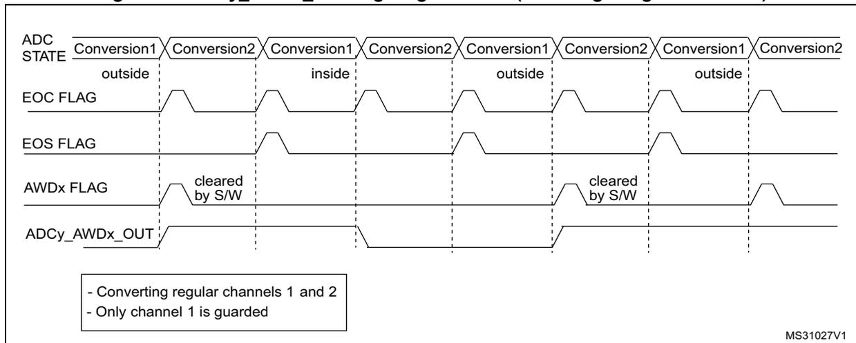
Figure 94. ADCy\_AWDx\_OUT signal generation (on all injected channels)
