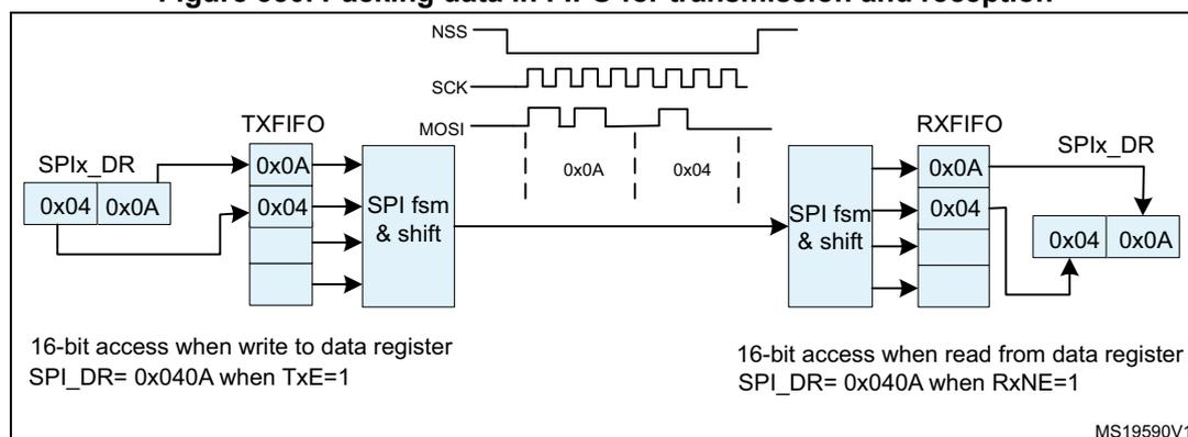
1. In this example: Data size DS[3:0] is 4-bit configured, CPOL=0, CPHA=1 and LSBFIRST =0. The Data storage is always right aligned while the valid bits are performed on the bus only, the content of LSB byte goes first on the bus, the unused bits are not taken into account on the transmitter side and padded by zeros at the receiver side.
