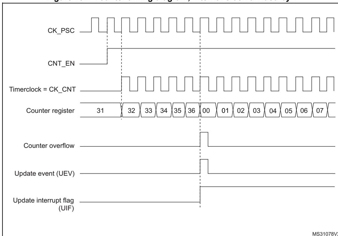
**Figure 193. Counter timing diagram, internal clock divided by 2**
