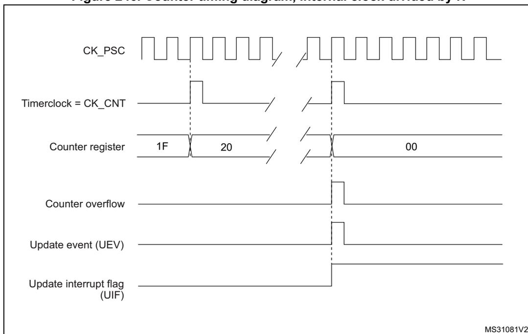
**Figure 247. Counter timing diagram, update event when ARPE=0 (TIMx\_ARR not preloaded)**
