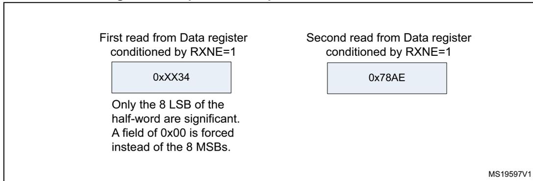
**Figure 372. LSB justified 16-bit extended to 32-bit packet frame**
