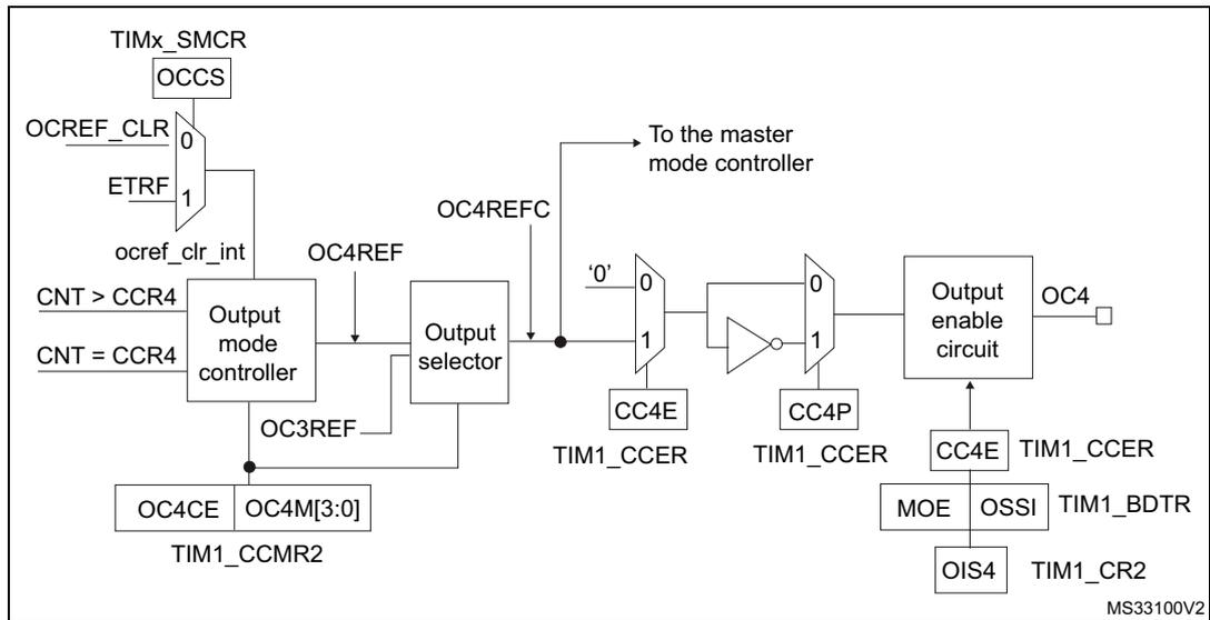
Figure 163. Output stage of capture/compare channel (channel 5, idem ch. 6)
