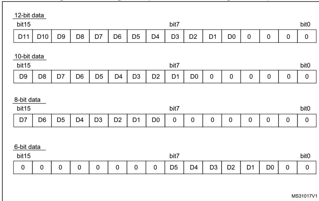
**Figure 83. Left alignment (offset enabled, signed value)**
