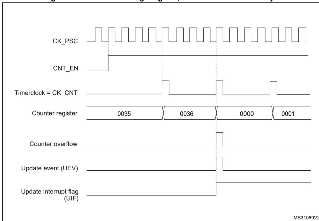
Figure 246. Counter timing diagram, internal clock divided by N
