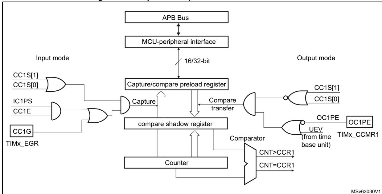
Figure 216. Output stage of Capture/Compare channel (channel 1)
