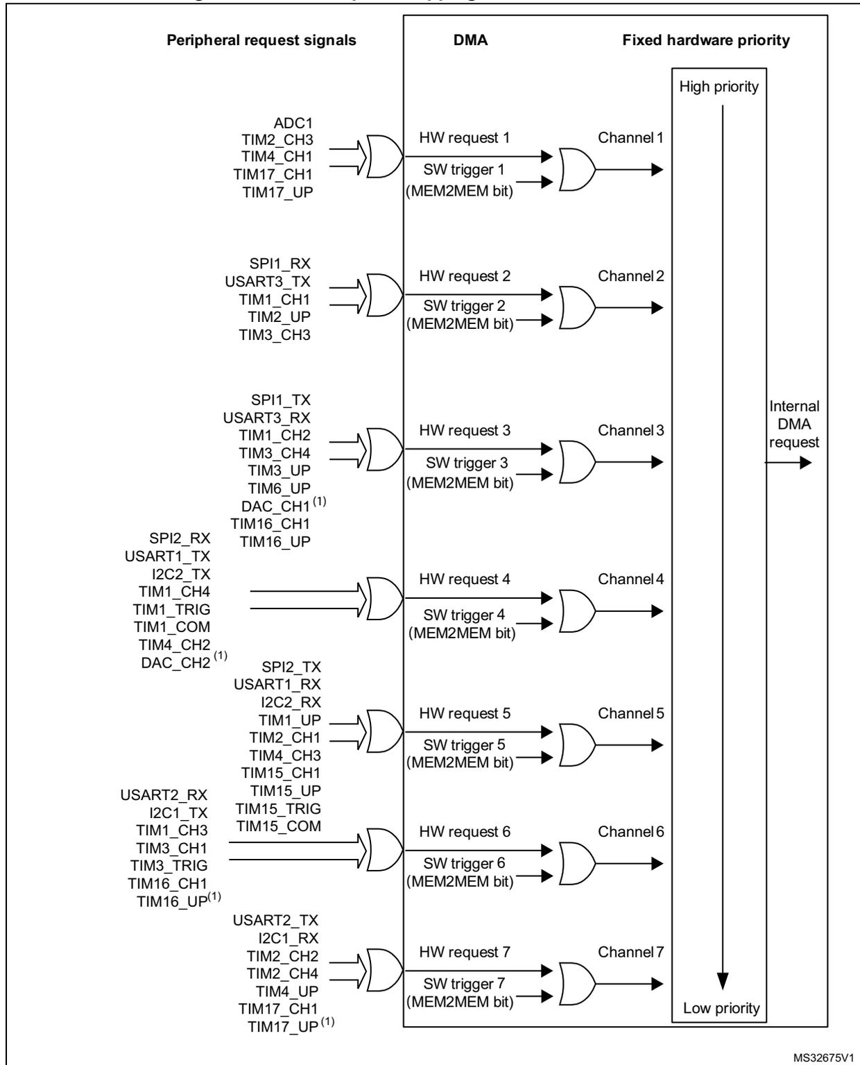
1. DMA request mapped on this DMA channel only if the corresponding remapping bit is set in *SYSCFG configuration register 1 (SYSCFG\_CFGR1)*.
