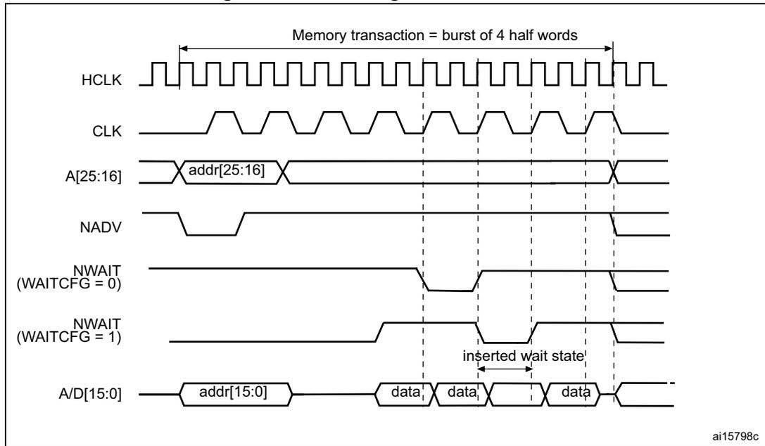
Figure 47. Synchronous multiplexed read mode waveforms - NOR, PSRAM (CRAM)
