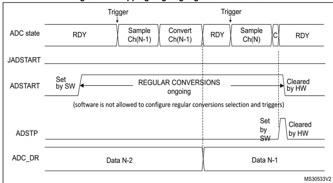
Figure 60. Stopping ongoing regular and injected conversions
