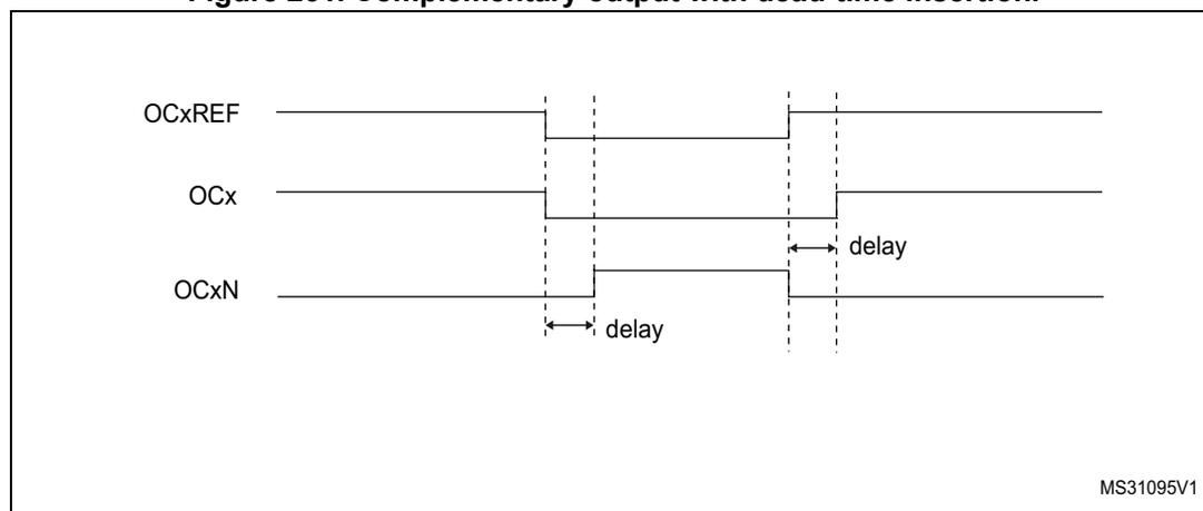
**Figure 262. Dead-time waveforms with delay greater than the negative pulse.**
