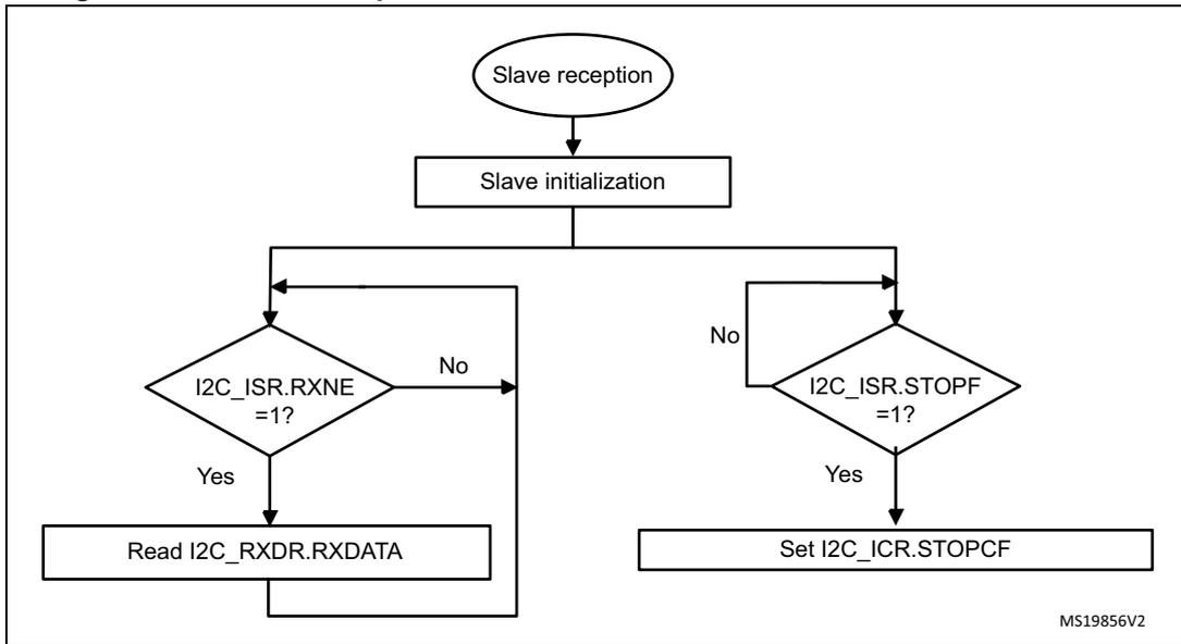
Figure 298. Transfer bus diagrams for I2C slave receiver
