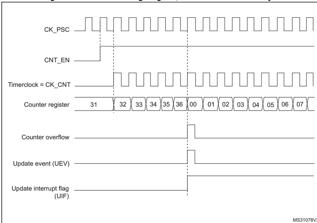
Figure 244. Counter timing diagram, internal clock divided by 2
