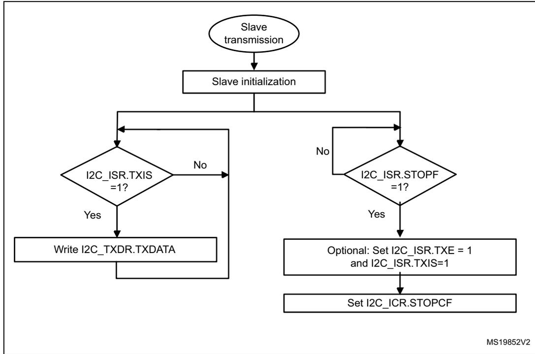
Figure 295. Transfer bus diagrams for I2C slave transmitter
