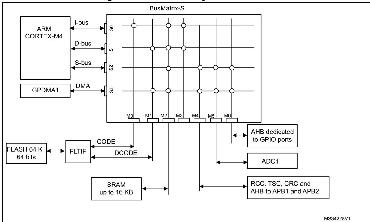
Figure 3. STM32F302xD/E system architecture
