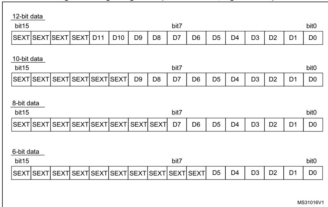
**Figure 82. Left alignment (offset disabled, unsigned value)**
