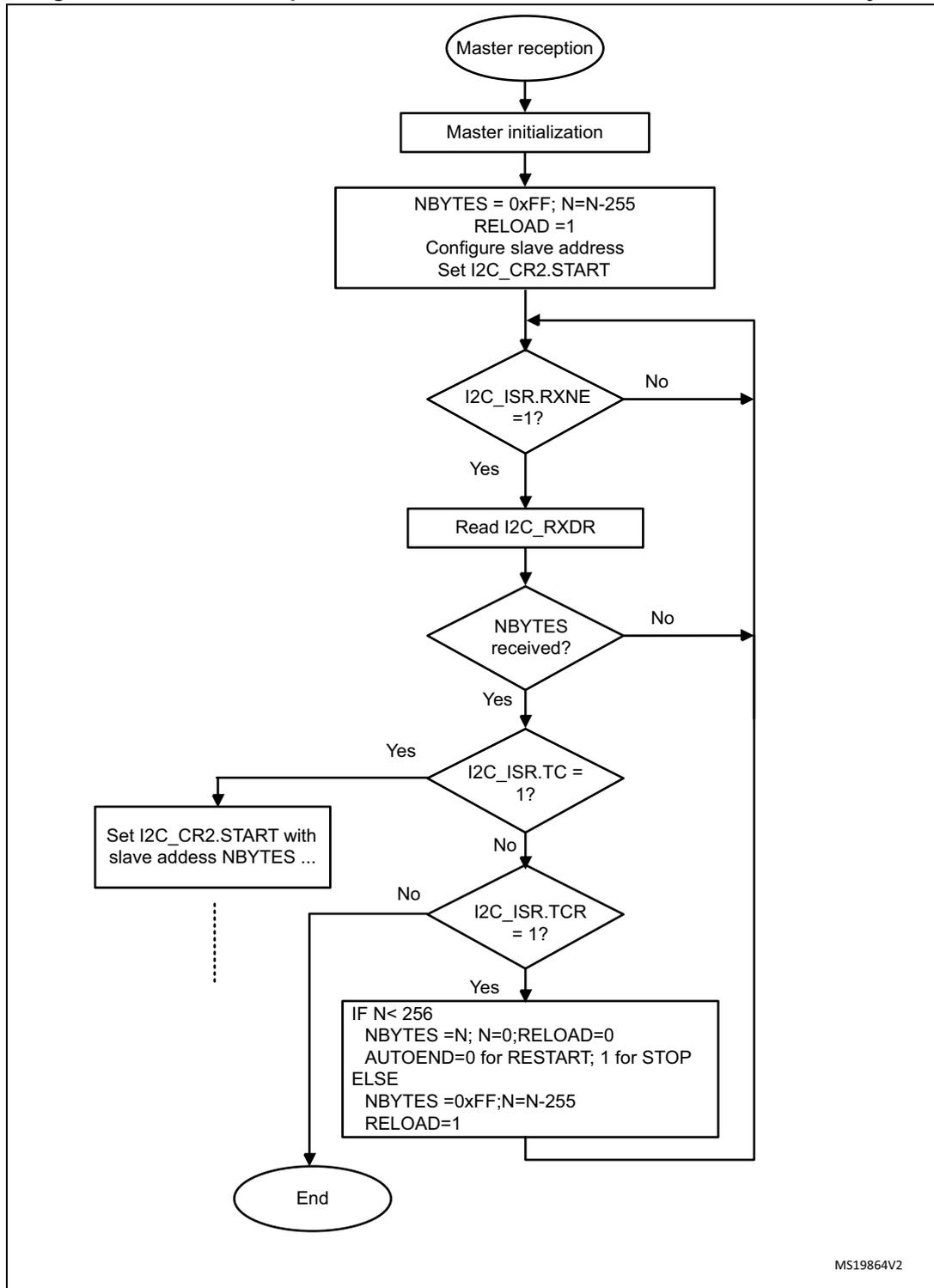
Figure 308. Transfer bus diagrams for I2C master receiver
