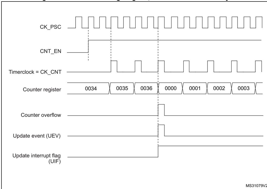
Figure 245. Counter timing diagram, internal clock divided by 4
