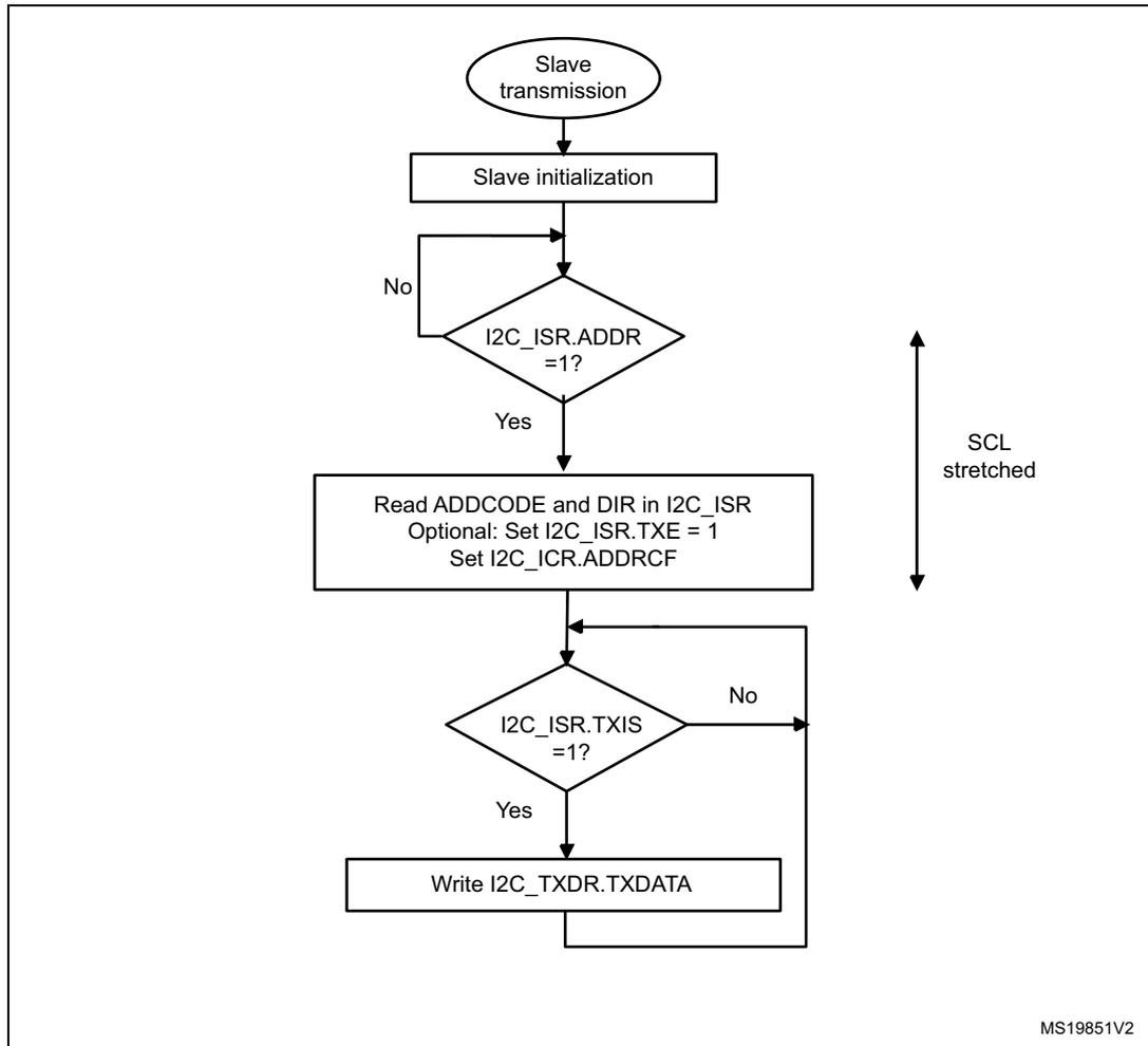
Figure 294. Transfer sequence flowchart for I2C slave transmitter, NOSTRETCH= 1
