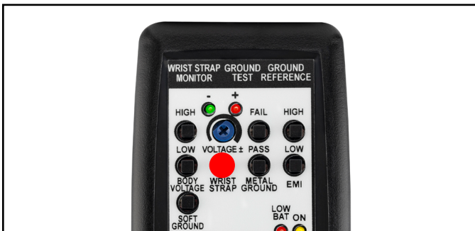
Figure 4. Pressing the WRIST STRAP test switch
