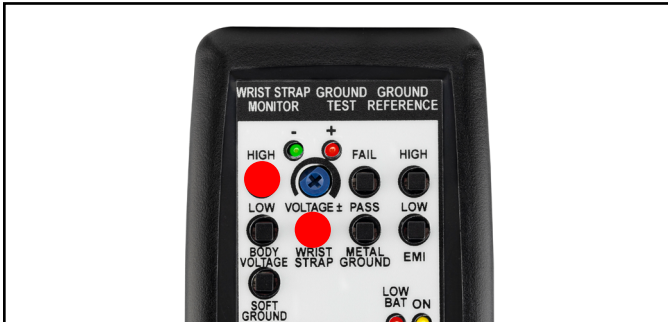
Figure 12. Pressing the WRIST STRAP and HIGH BODY VOLTAGE test switches simultaneously
