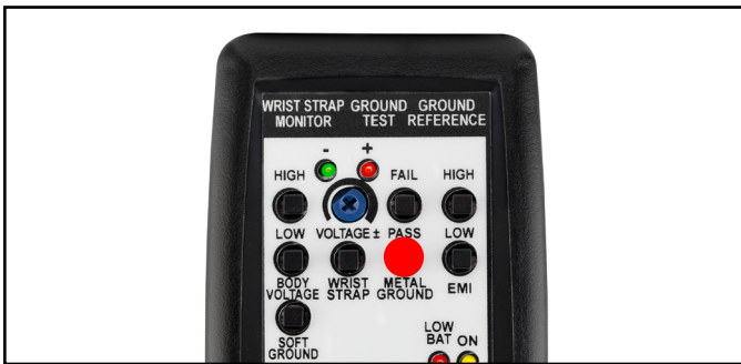
Figure 30. Pressing the METAL GROUND PASS test switch
