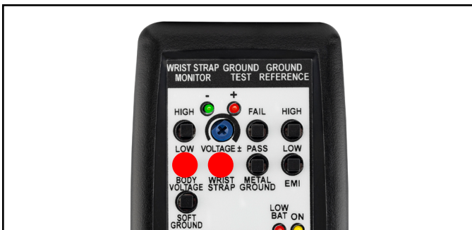
Figure 5. Pressing the WRIST STRAP and LOW BODY VOLTAGE test switches simultaneously
