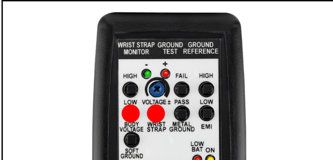
Figure 11. Pressing the WRIST STRAP and LOW BODY VOLTAGE test switches simultaneously
