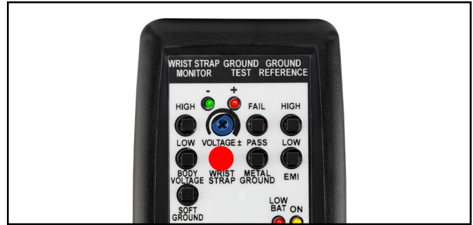
Figure 26. Pressing the WRIST STRAP test switch
