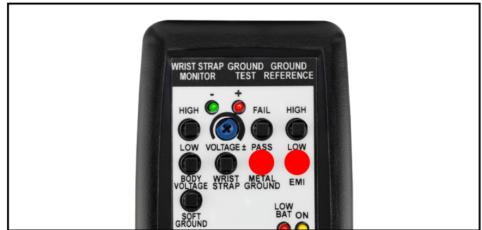
Figure 32. Pressing the METAL GROUND PASS and EMI LOW test switches simultaneously
