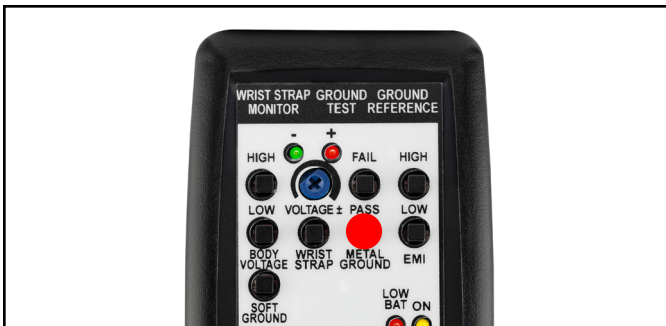
Figure 21. Pressing the METAL GROUND PASS test switch
