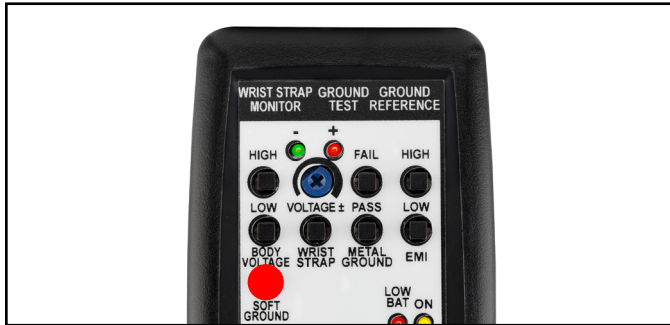
Figure 8. Pressing the SOFT GROUND test switch
