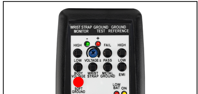
Figure 14. Pressing the SOFT GROUND test switch
