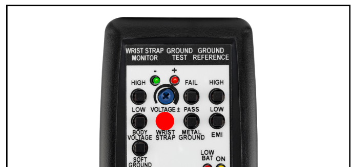
Figure 10. Pressing the WRIST STRAP test switch
