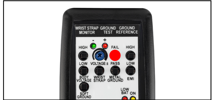
Figure 22. Pressing the METAL GROUND FAIL test switch
