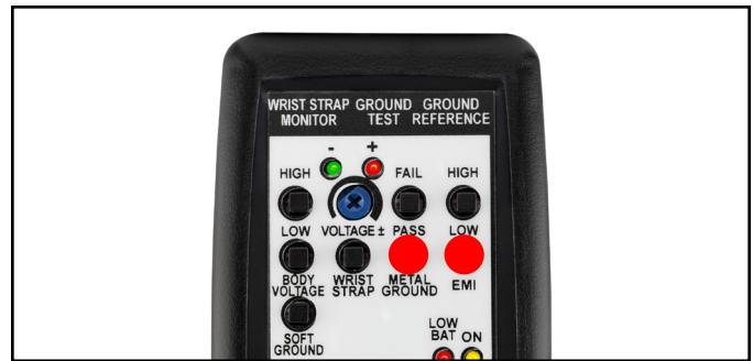
Figure 18. Pressing the METAL GROUND PASS and EMI LOW test switches simultaneously
