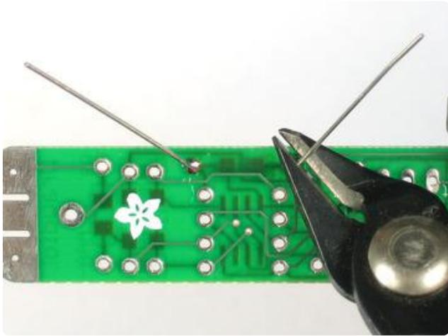
Using your diagonal cutters, cut off the long leads just above the solder joint.
