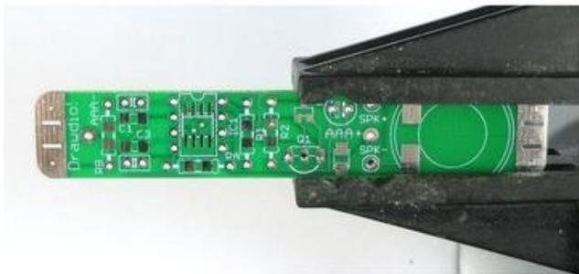
Get ready by placing the PCB in a vise.
