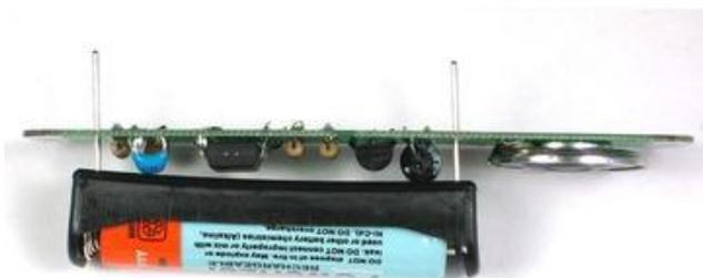
Slide the battery holder into the PCB (but do not solder it in). Make sure that the battery is aligned correctly. Putting in the battery backwards shouldn't damage the circuit but it's still not a good idea so try to get it right the first time. The back of the PCB has a silkscreen to help determine which way the battery goes in.
