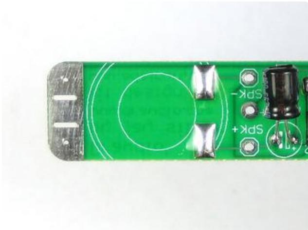
Now melt a lot of solder onto the two pads.
