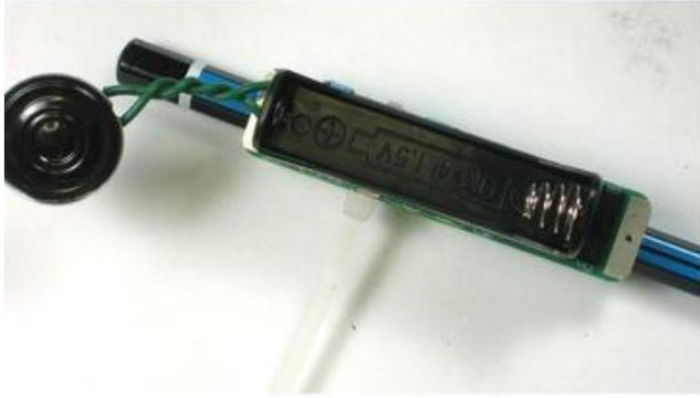
Next you can mount the PCB to your pencil. Place the PCB on the flat side of a pencil, and thread the zip tie through as shown and tighten it. You'll want it about an inch or less from the top of the pencil. The higher it is the more pencil you'll have to sharpen but it may be a little more unbalanced.
