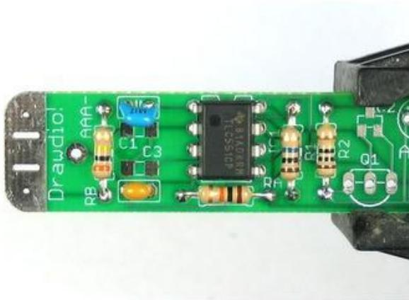
Next is the heart of the kit, a low voltage 555 timer chip. This one is called the TLC551. The important thing to note about the chip is that it is not symmetric. If it is put in wrong it will not work! Its also nearly impossible to fix if the chip goes in wrong so make triple-sure before you solder it in!
