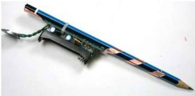
Finally, insert a battery into the kit. Then grip the pencil with one hand and touch the point of the pencil to your other hand. You will be able to hear the drawdio make noise!
