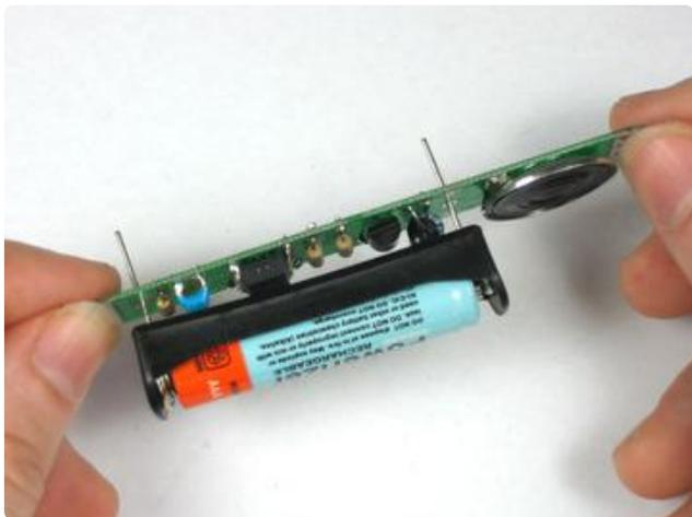
With the battery holder in place (but, again, not soldered in) touch both sides of the PCB. A squeaking noise should come out of the speaker! As you press harder/softer, the pitch will change. That indicates the circuit is working.
