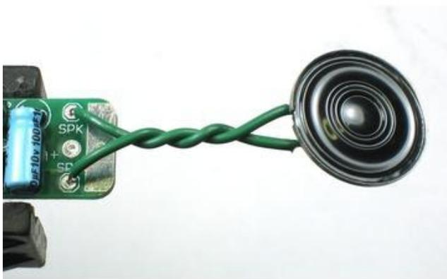
Twist the wires, this will reduce the strain on the solder joints when bending. Put the end of each wire into the two PCB holes marked SPK+ and SPK-. Don't solder into the hole in the middle which is for the battery. The speaker is 'symmetric' so it doesn't matter which wire goes in which hole.
