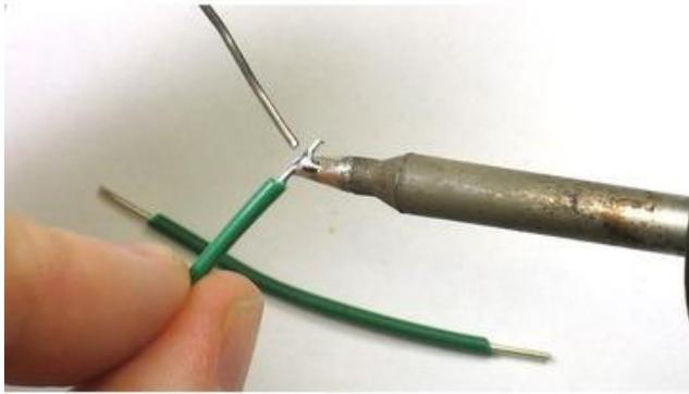
Next, it is a good idea to tin the ends of the wires. Its a little tricky because it requires holding three things. However, if you have a 'third hand tool' or a vise, you can use that to hold the wire while you heat up the stripped end and coat it with a little bit of solder. This will make it easier to connect to the speaker.
