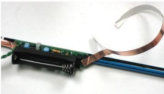
Next take 3 or 4" of copper tape and start wrapping around the bottom of the pencil, starting with the silver tab on the PCB and ending an inch before the end of the pencil. This will make contact with your hand and provide the second half of the sensor.
