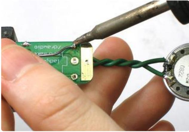
Solder the wires into place.
