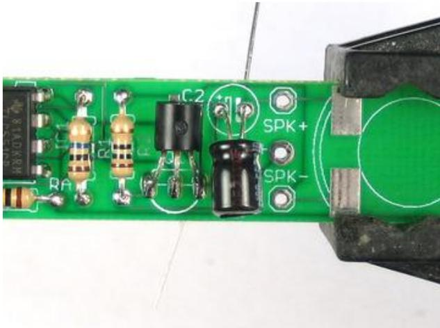
Fold the capacitor down so that it lies flat against the PCB.
