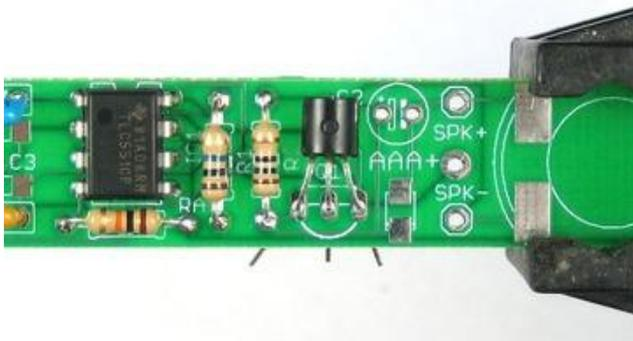
Now bend over the transistor so its 'face flat' against the PCB.
