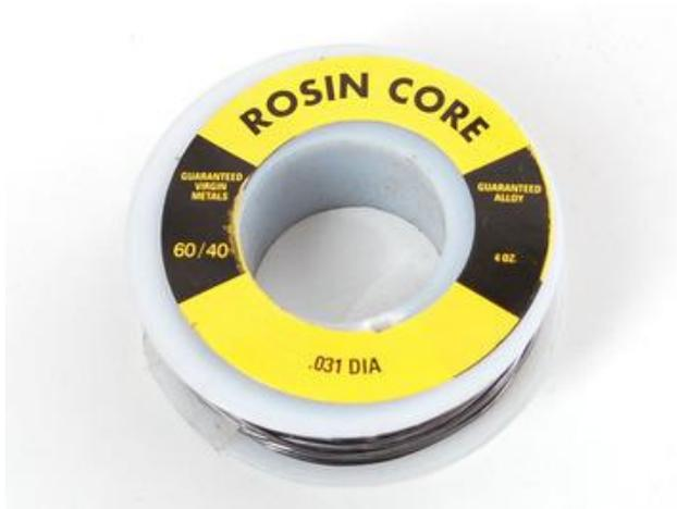
You will want rosin core, 60/40 solder. Good solder is a good thing. Bad solder leads to bridging and cold solder joints which can be tough to find.
