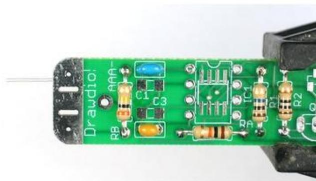
C3 is a yellow 0.1uF capacitor and has a "104" marking on it. C1 is the blue or orange 680pF capacitor and has a "681" marking on it.
