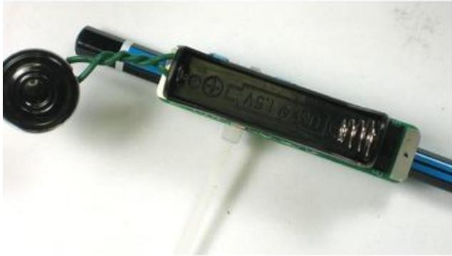
You can mount the drawdio to your pencil. Place the PCB on the flat side of a pencil, and thread the zip tie through as shown and tighten it. You'll want it about an inch or less from the top of the pencil. The higher it is the more pencil you'll have to sharpen but it may be a little more unbalanced.
