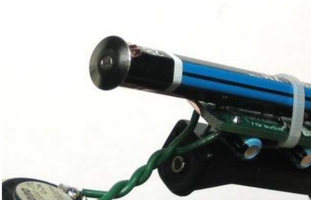
Then take the thumbtack and gently push it into the end of the pencil. You might have to twist it back & forth a little to get it all the way in. The thumbtack will grip the copper tape and also make contact with the graphite in the middle of the pencil to make the first half of the drawing sensor.
