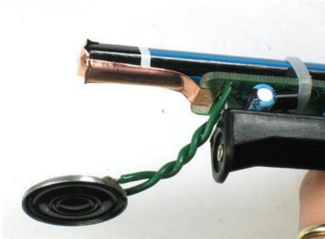
Wrap the tape along the top of the pencil so that the beginning is at the silver metal tab on the PCB, as shown.
