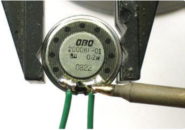
Next, warm up the tabs and slide the tinned ends of wire into the melted solder pool. Then remove the iron and wait a few seconds, the solder pool will cool with the wire in place. Do the same for the other pad.
