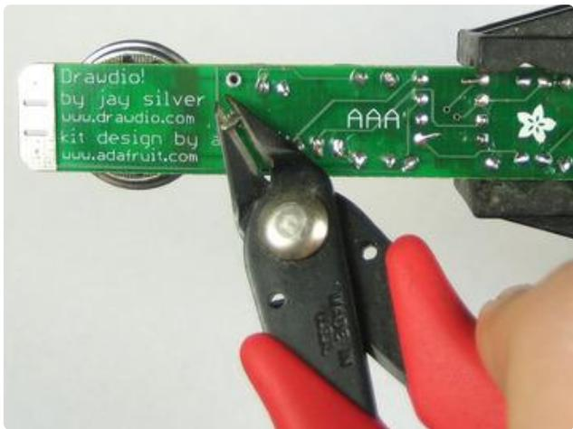
Solder in the battery holder, and clip the leads short.
