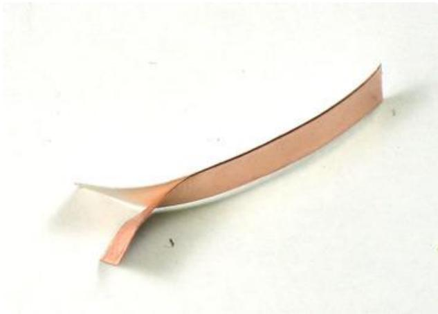
Next cut a 1.5" piece of copper tape using the diagonal cutters. Don't use scissors as the metal tape can damage them. Peel off the paper backing. The copper tape is conductive, sticky and flexible which makes it perfect for wrapping the pencil.
