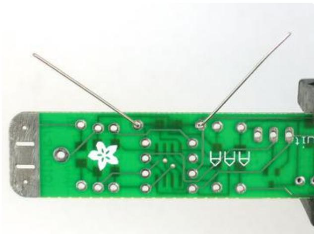
Place the resistor in the location marked RA. Resistors do not have polarity which means you can put it in 'either way' and it will work just fine. Bend the wire legs out so that the resistor sits flat against the PCB.
