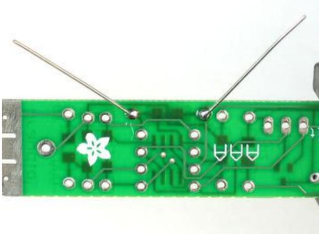
Turn the PCB over. Using your soldering iron tip, press and heat both the pad (the silver ring around the hole) and lead (wire) at the same time for 2 or 3 seconds. Then poke the end of the solder in to create a nice solder joint. Do this for both leads.
