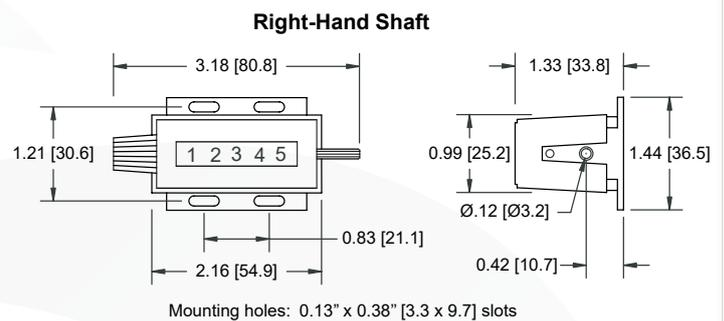
A compact, 5 figure, rotary counter, indicating 10 counts/revolution. Design and compact size make it ideally suited for office and test equipment, coin counting and other direct reading instruments.
