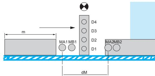
D1, D2, D3, D4: monitoring photo-electric sensors.
