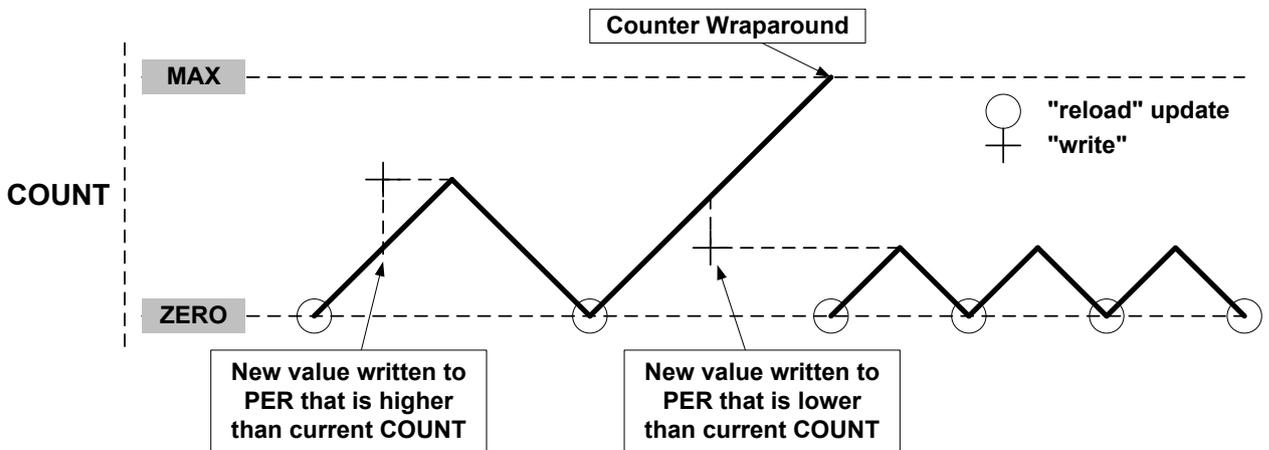
When double buffering is used, the buffer can be written at any time and the counter will still maintain correct operation. The period register is always updated on the update condition, as shown in [Figure 31-13](#). This prevents wraparound and the generation of odd waveforms.
