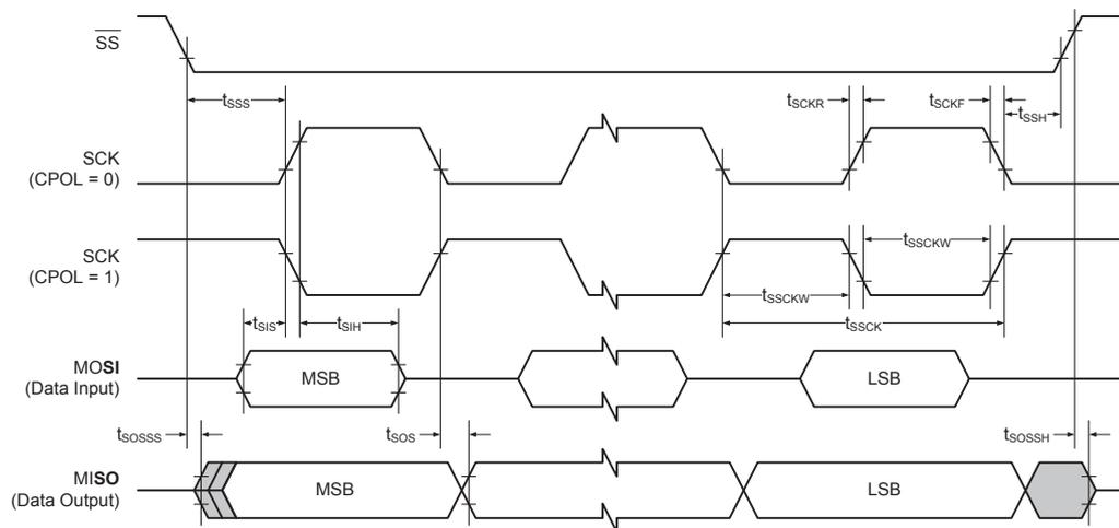
**Table 37-59. SPI Timing Characteristics and Requirements<sup>(1)</sup>**
