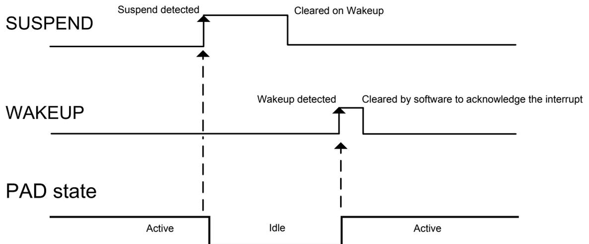
The Suspend Interrupt bit in the Device Interrupt Flag register (INTFLAG.SUSPEND) is set when a USB Suspend state has been detected on the USB bus. The USB pad is then automatically put in the Idle state. The detection of a non-idle state sets the Wake Up Interrupt bit in INTFLAG (INTFLAG.WAKEUP) and wakes the USB pad.
