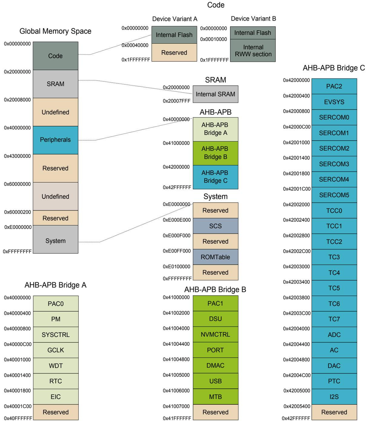
This figure represents the full configuration of the Atmel® SAM D21 with maximum flash and SRAM capabilities and a full set of peripherals. Refer to the [Configuration Summary](#) for details.
