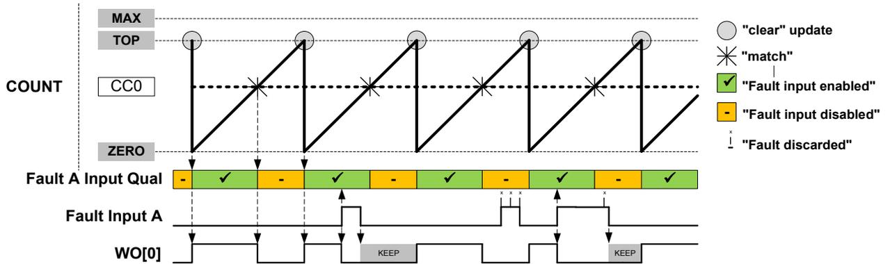
**Restart Action** This is enabled by writing the Fault n Restart bit in Recoverable Fault n Configuration register (FCTRLn.RESTART) to '1'. When enabled, the timer/counter will be restarted as soon as the corresponding fault condition is present. The ongoing cycle is stopped and the timer/counter starts a new cycle, see Figure 31-24. In Ramp 1 mode, when the new cycle starts, the compare outputs will be clamped to inactive level as long as the fault condition is present.
