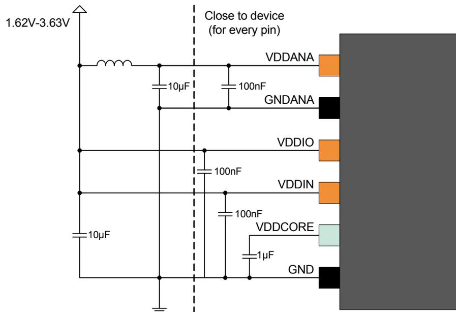
**Table 39-1. Power Supply Connections,  $V_{DDCORE}$  From Internal Regulator**
