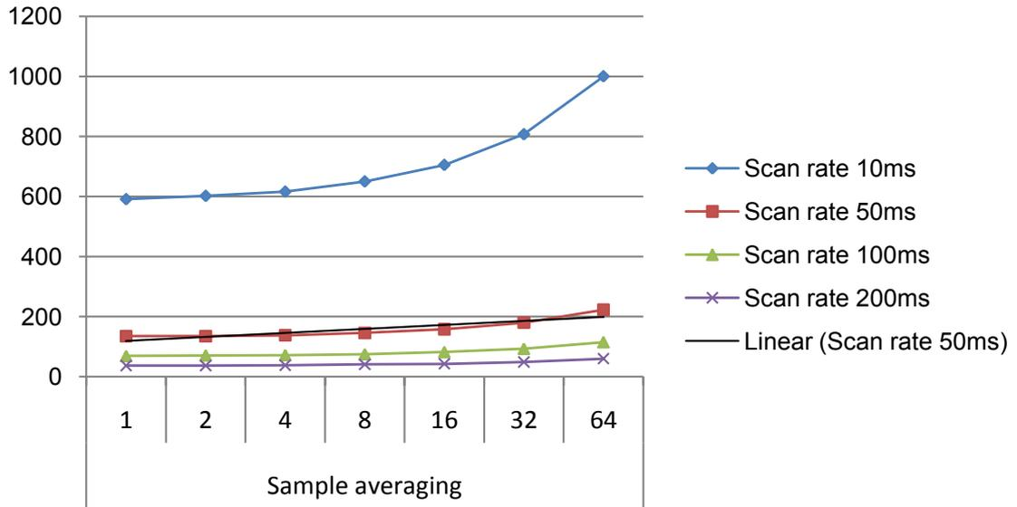
**Figure 37-10. Power Consumption [ $\mu$ A]**
