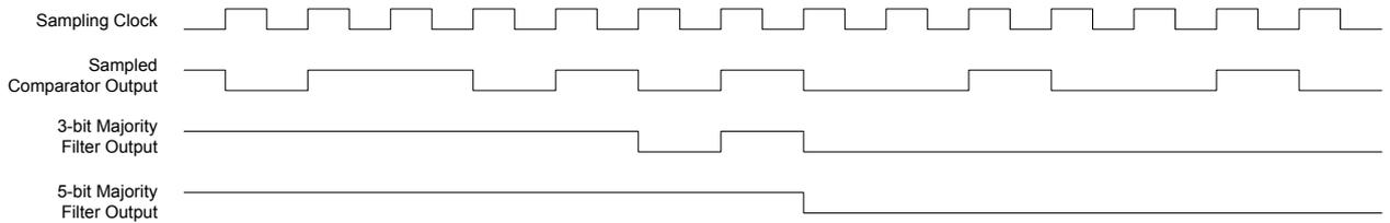
**Figure 34-7. Single-Shot Filtering**
