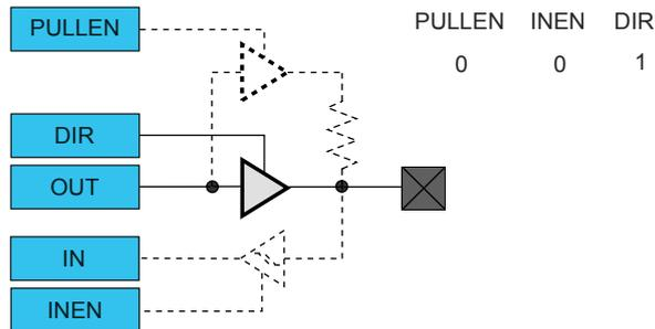
Figure 23-7. I/O Configuration - Totem-Pole Output with Enabled Input
