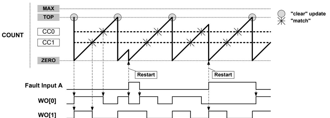
relative local Minimum (for CAPTMIN) or Maximum (for CAPTMAX) value has been detected. DERIV0 is equivalent to an OR function of (LOCMIN, LOCMAX).
