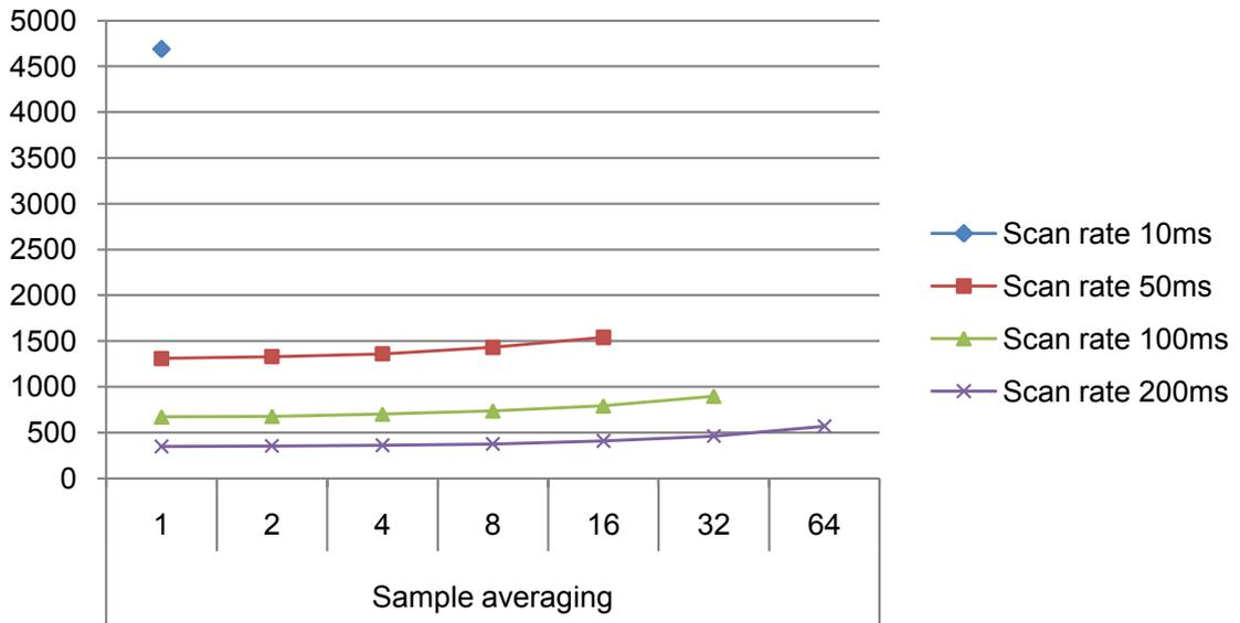
**Figure 37-12. Power Consumption [ $\mu$ A]**
