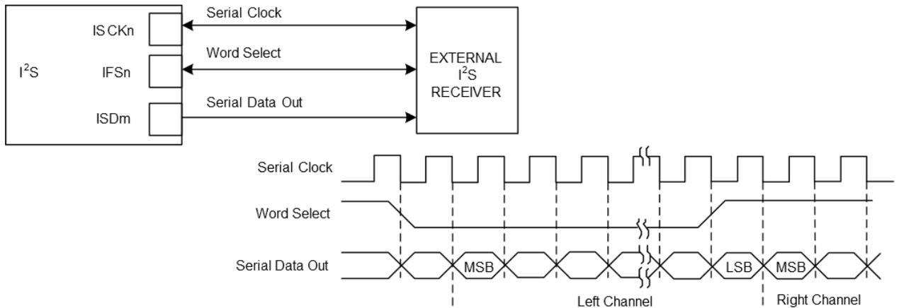
**Figure 29-8. Time Slot Application Block Diagram**
