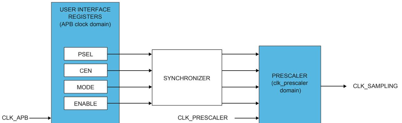
The BOD33 Clock Enable bit (BOD33.CEN) in the BOD33 register and the BOD12 Clock Enable bit (BOD12.CEN) in the BOD12 register should always be disabled before changing the prescaler value. To change the prescaler value for the BOD33 or BOD12 during sampling mode, the following steps need to be taken:
