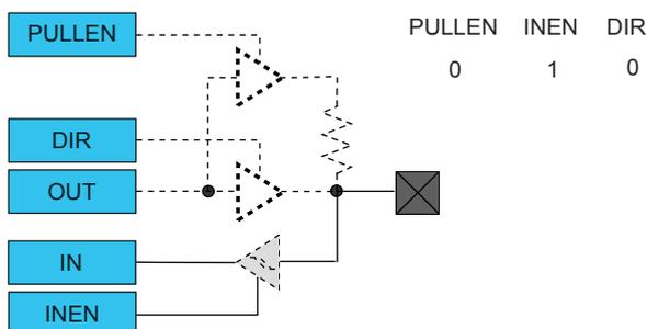
Figure 23-5. I/O Configuration - Input with Pull
