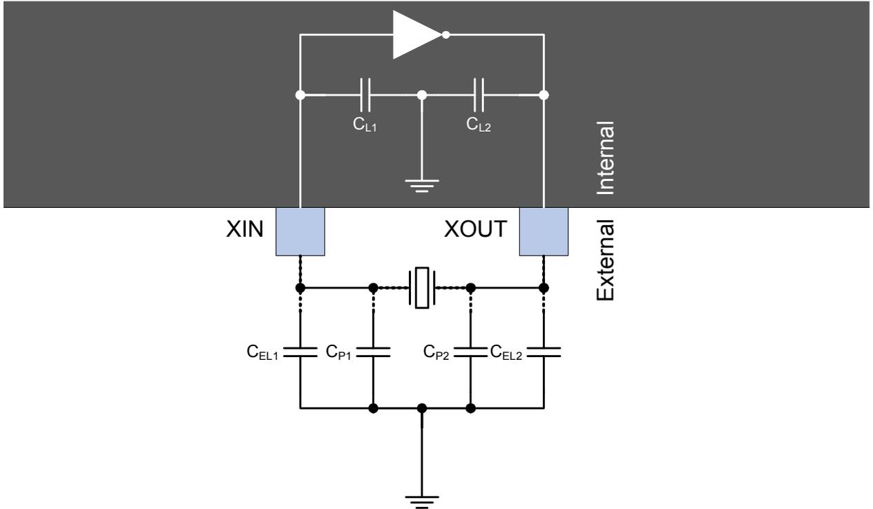
Using this model the total capacitive load for the crystal can be calculated as shown in the equation below:
