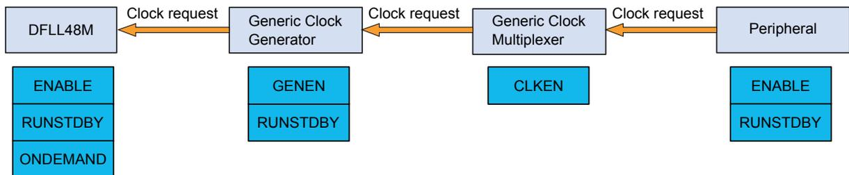
All clock sources in the system can be run in an on-demand mode: the clock source is in a stopped state unless a peripheral is requesting the clock source. Clock requests propagate from the peripheral, via the GCLK, to the clock source. If one or more peripheral is using a clock source, the clock source will be started/kept running. As soon as the clock source is no longer needed and no peripheral has an active request, the clock source will be stopped until requested again.
