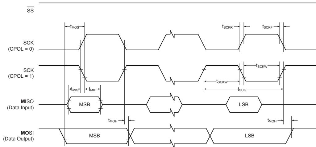
Figure 37-21. SPI Timing Requirements in Slave Mode
