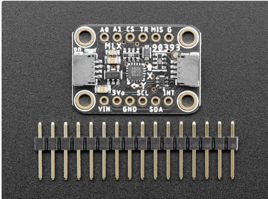
Comes as a fully assembled and tested breakout board with a small piece of header for use with a breadboard. As if that weren't enough, we've now also added [SparkFun qwiic \(\)](#) compatible [STEMMA QT \(\)](#) connectors for the I2C bus so you don't even need to solder the I2C and power lines. Just wire up to your favorite micro using a [STEMMA QT adapter cable. \(\)](#) The Stemma QT connectors also mean the MLX90393 can be
