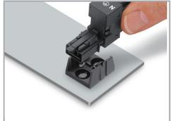
Secure the mounting plate via pins.
