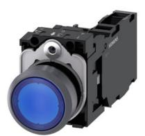
Illuminated pushbutton, 22 mm, round, plastic with metal front ring, blue, pushbutton, flat, momentary contact type, with holder, 1 NO+1 NC, LED module with integrated LED 110 V AC, screw terminal, with laser labeling, upper case
