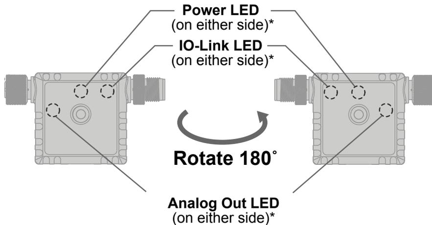
\* Indicator LEDs are visible through translucent housing
