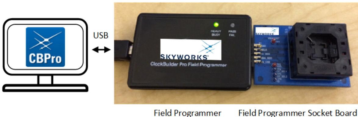
Figure 4.3. Connections from PC to the target device
