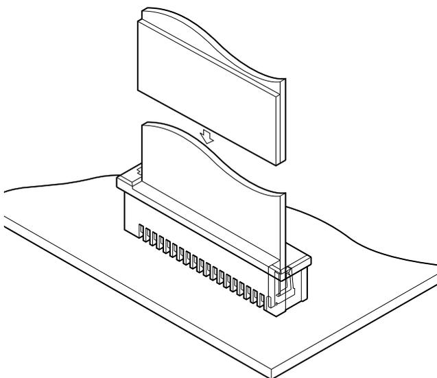
The FMZ series, a Zero Insertion Force (ZIF) connector series, was developed to increase wear resistance and extend the connector's mating life. It is a very compact connector with a thickness of only 4.2 mm and a pitch of only 1.0 mm and is thus useful for high density packaging. The contact has a reliable double-leaf construction which provides stable connection.
