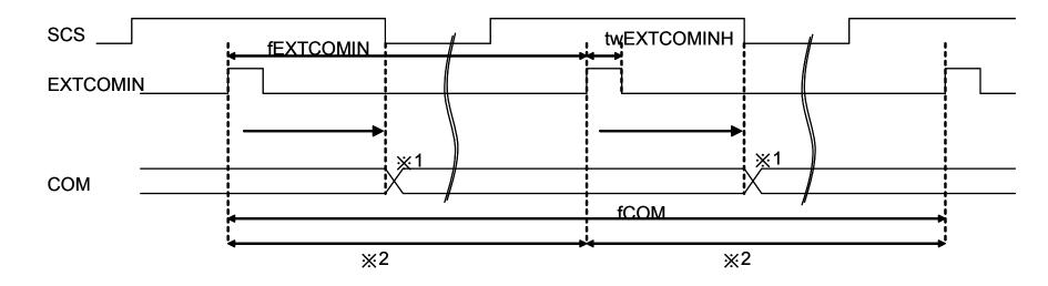
\* 1: LC inversion polarity has been set by the falling edge of SCS signal.
