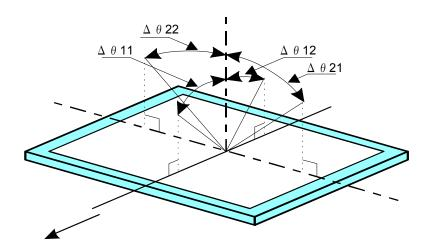
Figure 11-1 Definition of viewing angle direction
