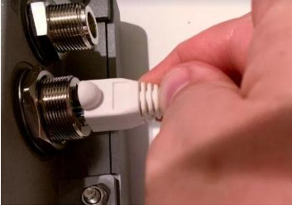
*Figure 6: Connecting the Ethernet cable to the gateway*
