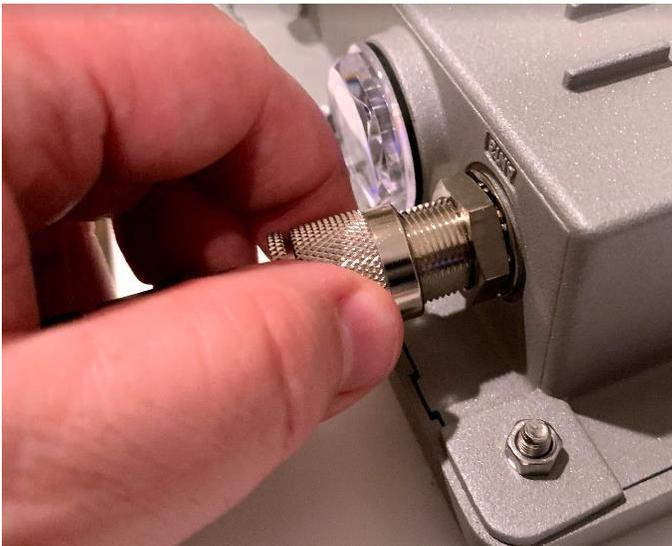
*Figure 5: Connecting the LoRa antenna to the gateway*
