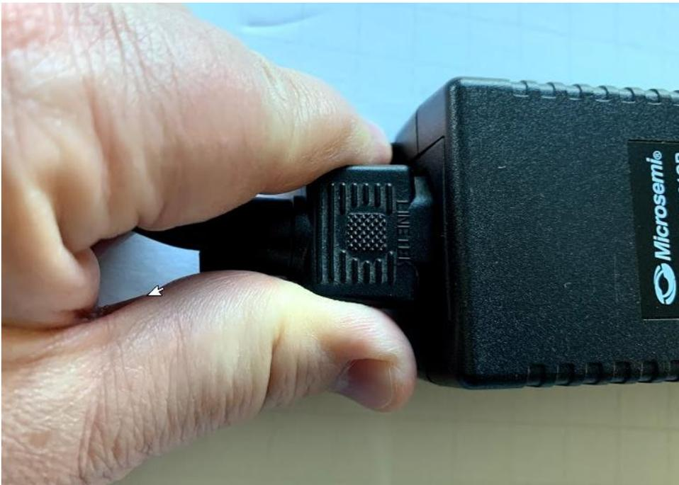
*Figure 11: Connecting mains cable to power brick*
