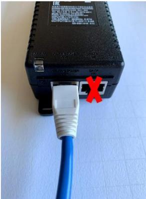
*Figure 7: Ethernet cable connected to the power brick*
