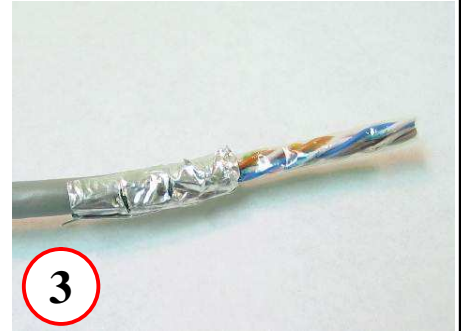
3 Fold back shield and drain wire
