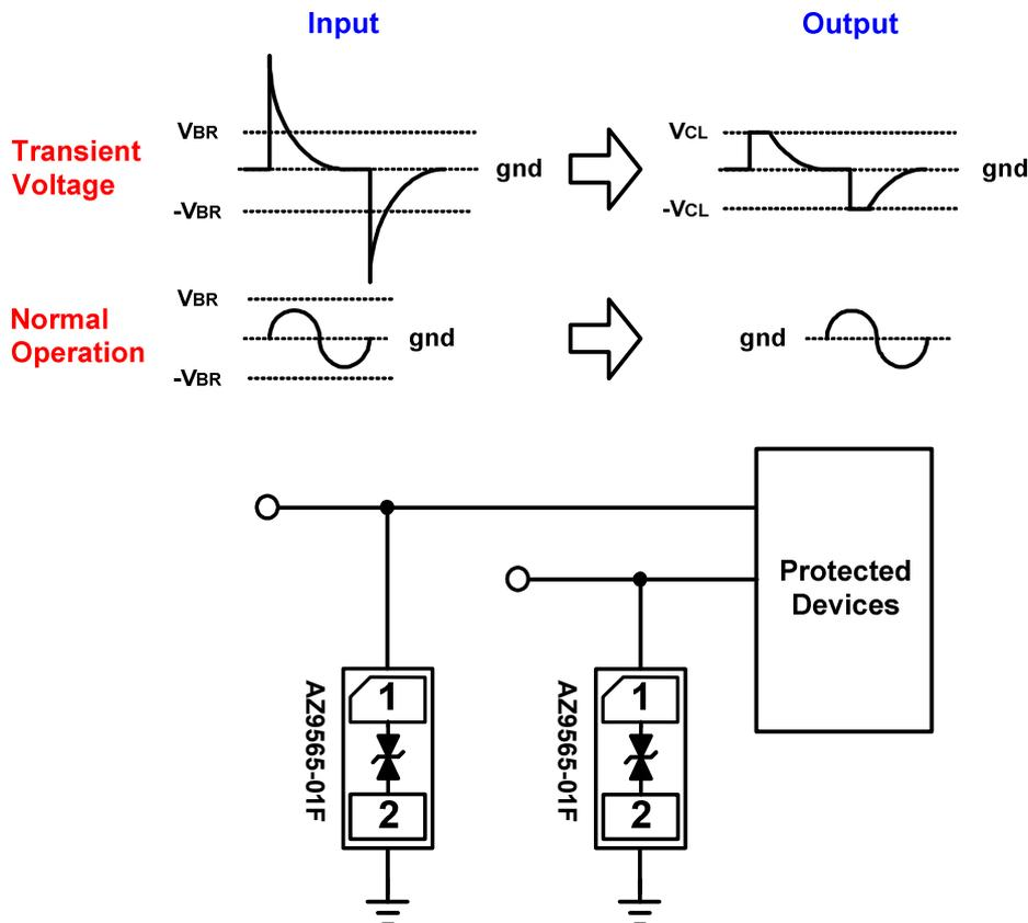
Fig. 1 ESD protection scheme by using AZ9565-01F.
