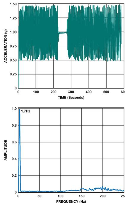
Figure 11. FFT Analysis on Acceleration Data Along the Z-Axis
