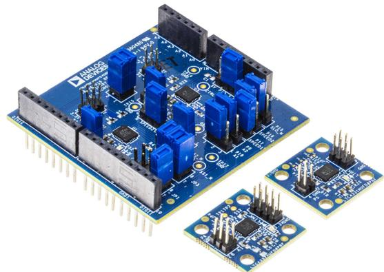
Figure 6. Local EVAL-CN0564-ARDZ Node and Remote Nodes of Both LTC4331 (I<sup>2</sup>C Extender) and LTC4332 (SPI Extender)
